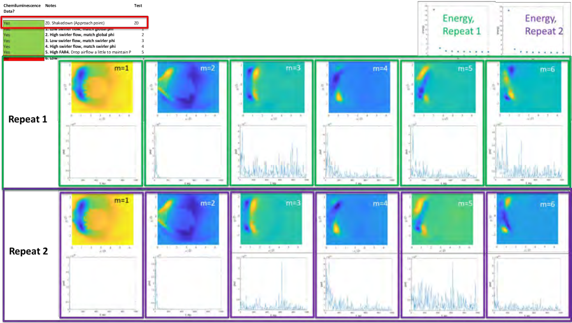
Figure 4. GT combustor repeatability study, baseline (Z0) approach condition.
