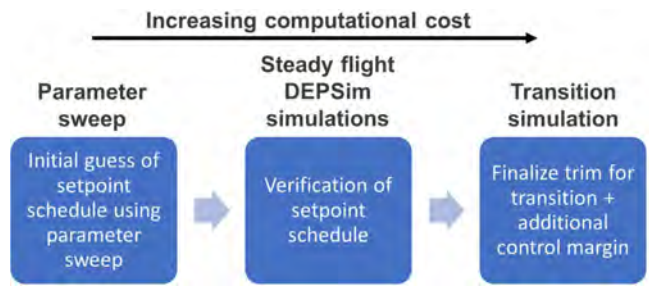
Figure 2. Strategy for building the rotor setpoint schedule (Mukherjee et al., 2023).
