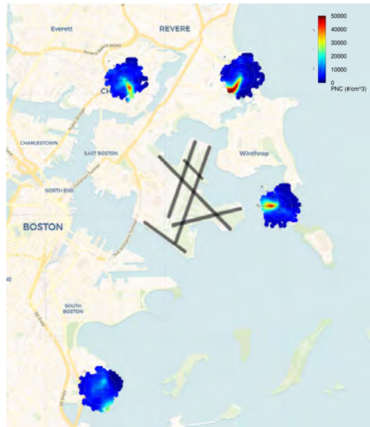
Figure 14. Polar plots of ultrafine particle number concentration (PNC) versus wind speed and direction at four sites near Logan Airport based on measurements from January 2021 to December 2022.
