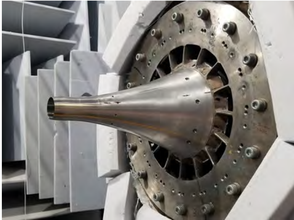
Figure 2. Primary nozzle from Gulfstream Aerospace Corporation with the baseline AXI mixer installed at the Georgia Tech Research Institute Anechoic Chamber.
