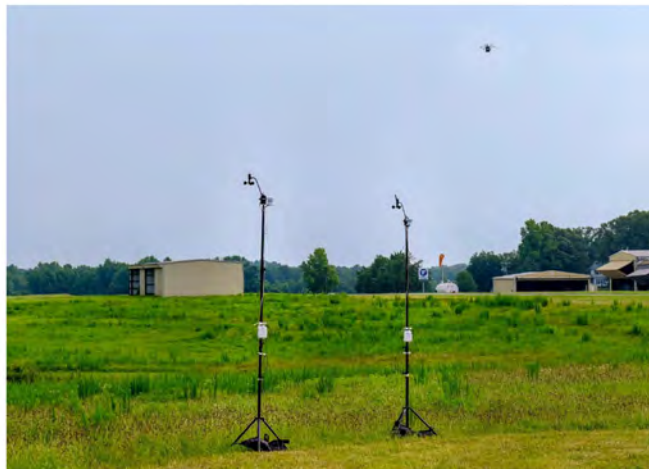
Figure 12. Anemometers for Weather data acquisition equipment.
