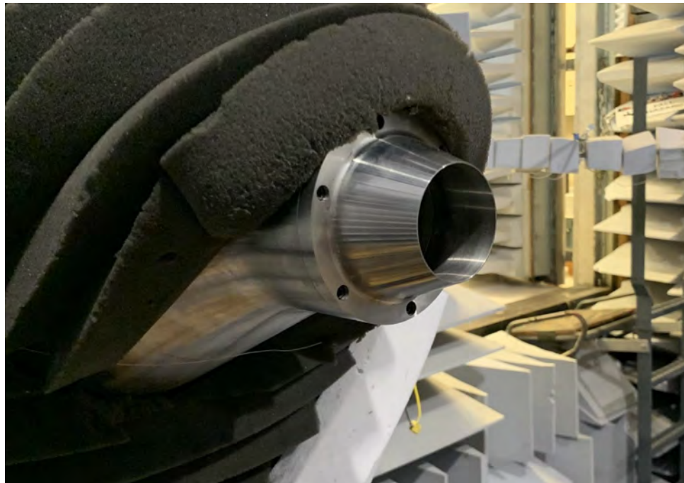
Figure 4. Full nozzle assembly from Gulfstream Aerospace Corporation at the Georgia Tech Research Institute Static Anechoic Chamber with an exhaust nozzle and mixing length of L_e/D_e = 1.0 .
