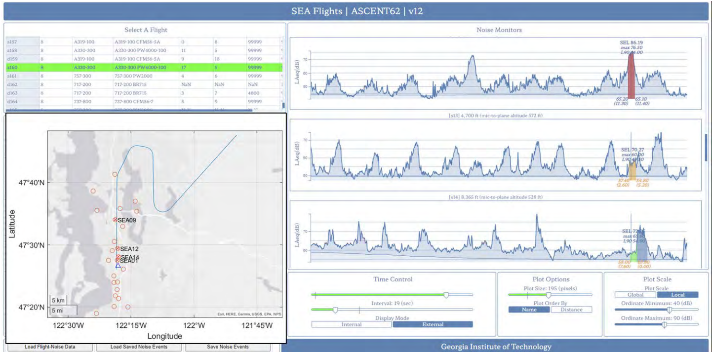
Figure 18. Developed dashboard to capture event sound exposure level (SEL) and maximum, A-weighted sound level ( L_{max} ) from Seattle-Tacoma International Airport (SEA) noise time history data
