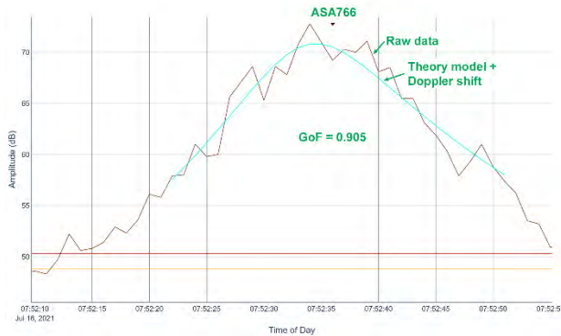
Figure 20. Example of the theoretical aircraft-peak model fit to a clean, raw sound peak recorded by the SFO sound monitor at NMT-12.
