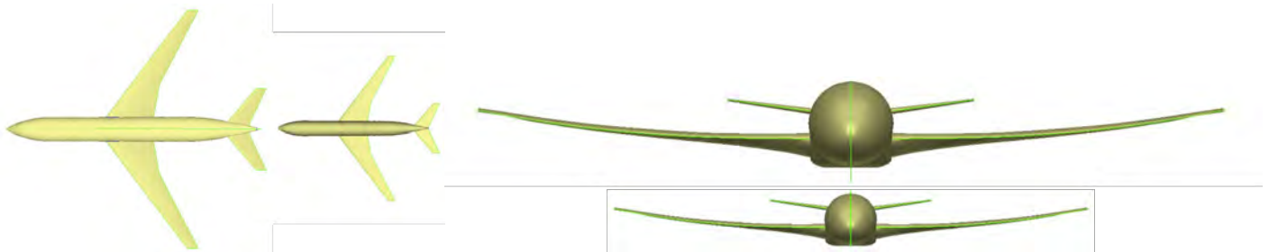
Figure 6. Side-by-side comparison of the Original NASA CRM aircraft and scaled-down version of the OWN baseline aircraft (modeled in ESP). Top view (Left) and front view (Right). The scale factor is 60.2% for the fuselage, 60.9% for the wing, and 62.25% for the horizontal tail (scaled with respect to longest dimension).
