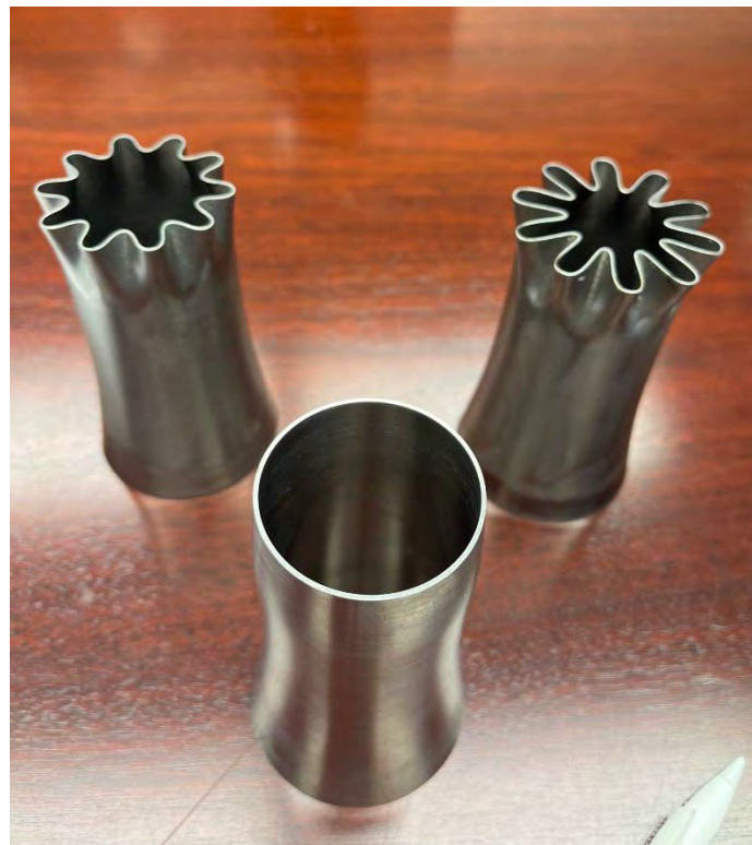
Figure 1. Three internal mixers for the ASCENT 59B Year 3 nozzle. Top left: SUN forced mixer. Top right: DAISY forced mixer. Bottom: AXI baseline mixer.
