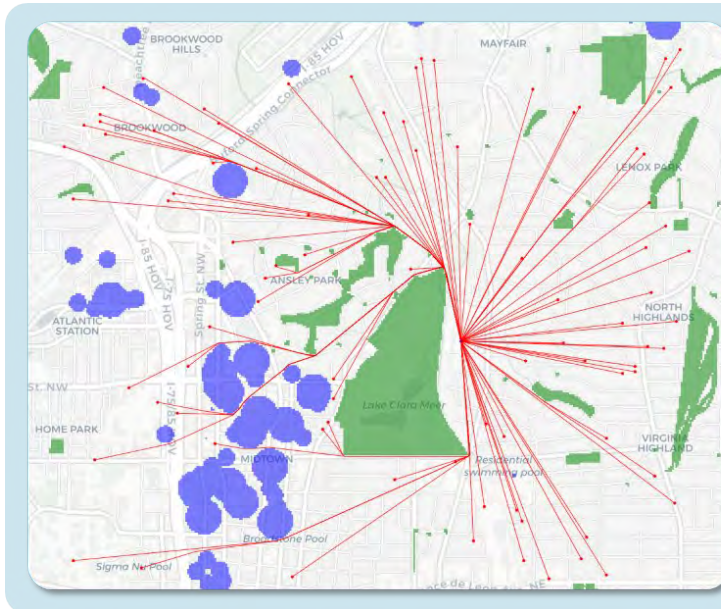
Figure 16. Example trajectories generated by the developed path planning logic. The study area under consideration is the Atlanta Midtown area.
