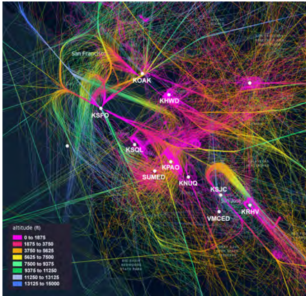
Figure 2. Typical daylong crowded traffic pattern in the SF metroplex (June 29, 2022). The flight path color codes indicate altitude range.
