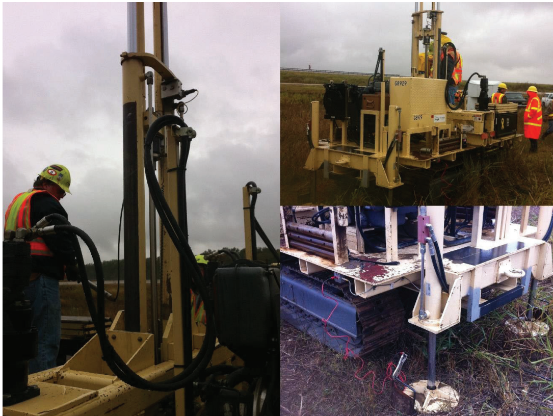
Figure 53. Images of the SCPT Equipment and Data Collection for the Turrell Site
