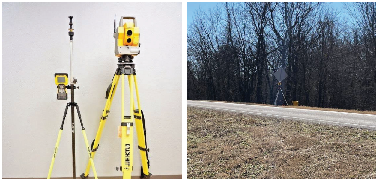
Figure 7. The Trimble 5600 DR200+ Robotic Total Station (left) and the Trimble Setup on Site (right)
