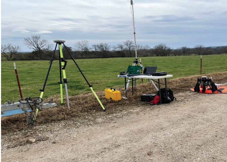
Figure 4. CHC 900 GNSS Base Station for LiDAR and Wifi Antenna
