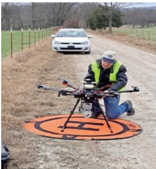
Figure 13. LiDAR and GNSS Being Setup for Lincoln Bridge 1 (East) (Job 040866)
