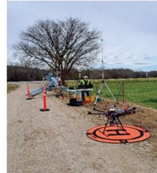
Figure 13. LiDAR and GNSS Being Setup for Lincoln Bridge 1 (East) (Job 040866)
