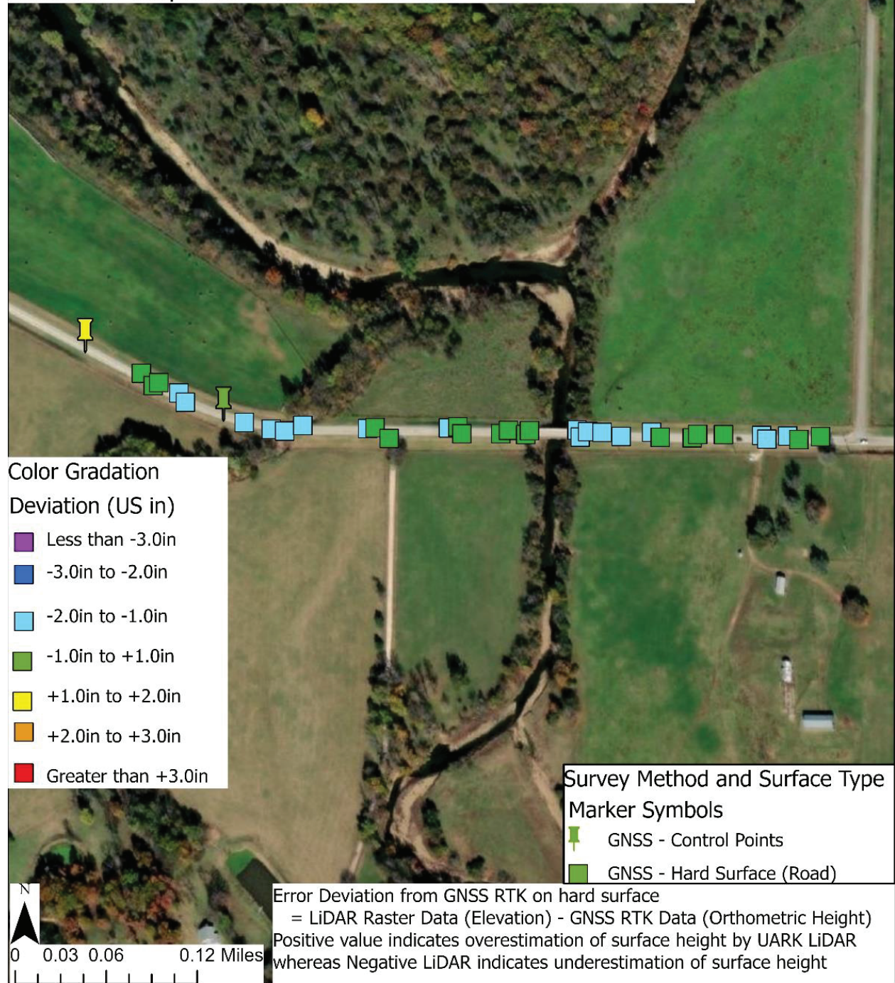
Figure 33. Aerial Image Showing the Comparison of UARK LiDAR Raster Elevations with GNSS Checkpoints for Hard Surfaces at Lincoln Bridge 1 (East) (Job 040866)
