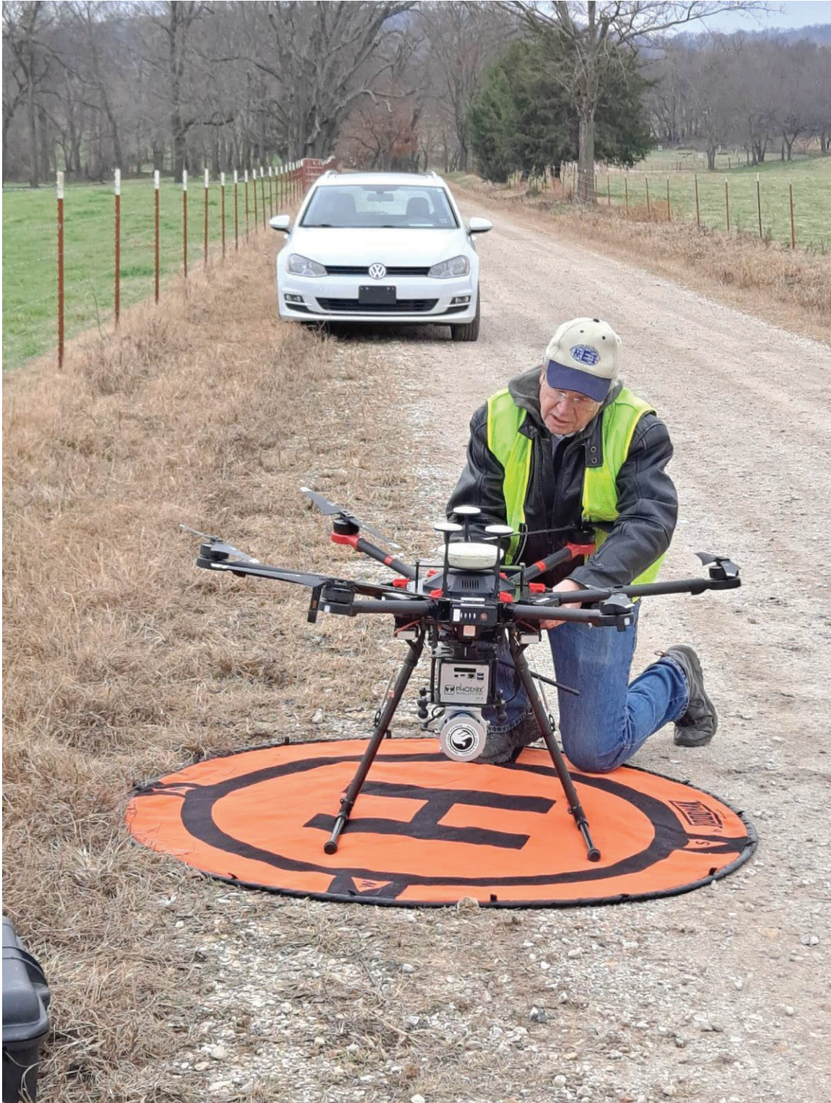
Figure 3. UAS and LiDAR Being Setup for Flight at the Site
