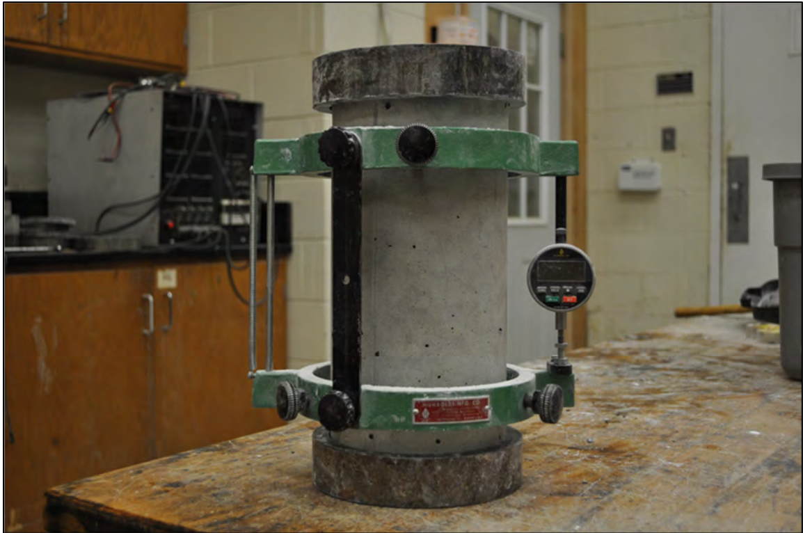
Figure 4-6: Compressometer used to test modulus of elasticity
