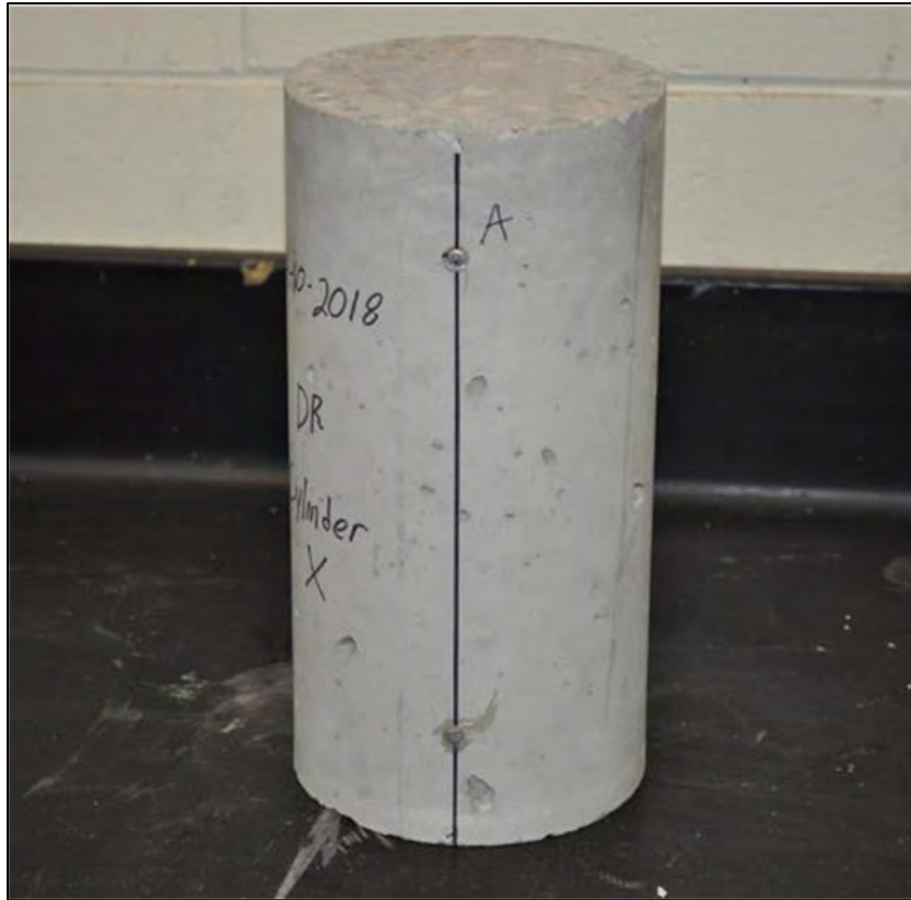
Figure 4-8: DEMEC points installed on shrinkage cylinder
