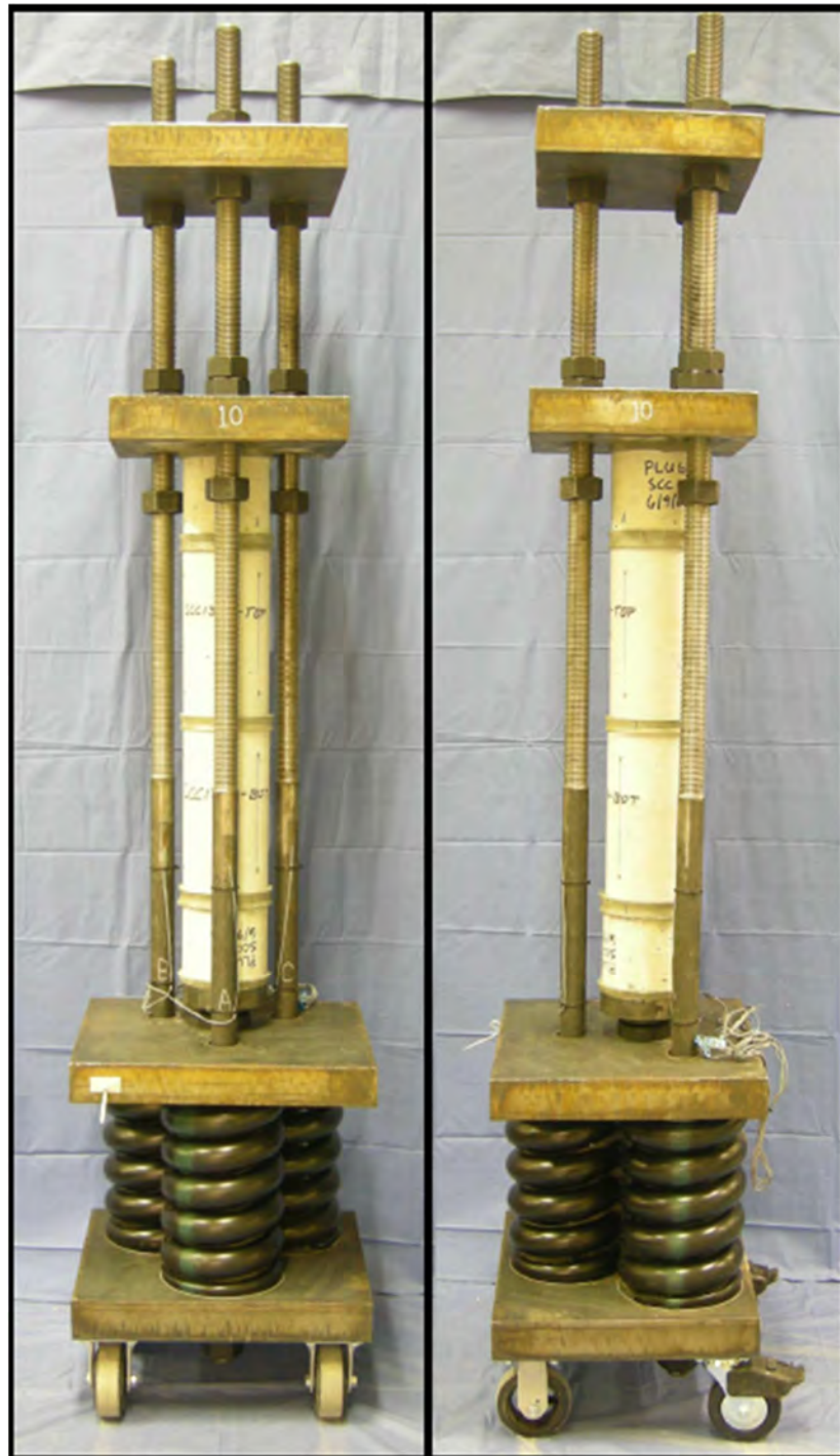
Figure 4-12: Creep testing frame (Kavanaugh 2008)
