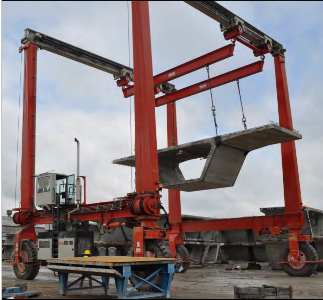
Figure 5-14: Rubber-tired gantry crane used to transport segments around the casting yard
