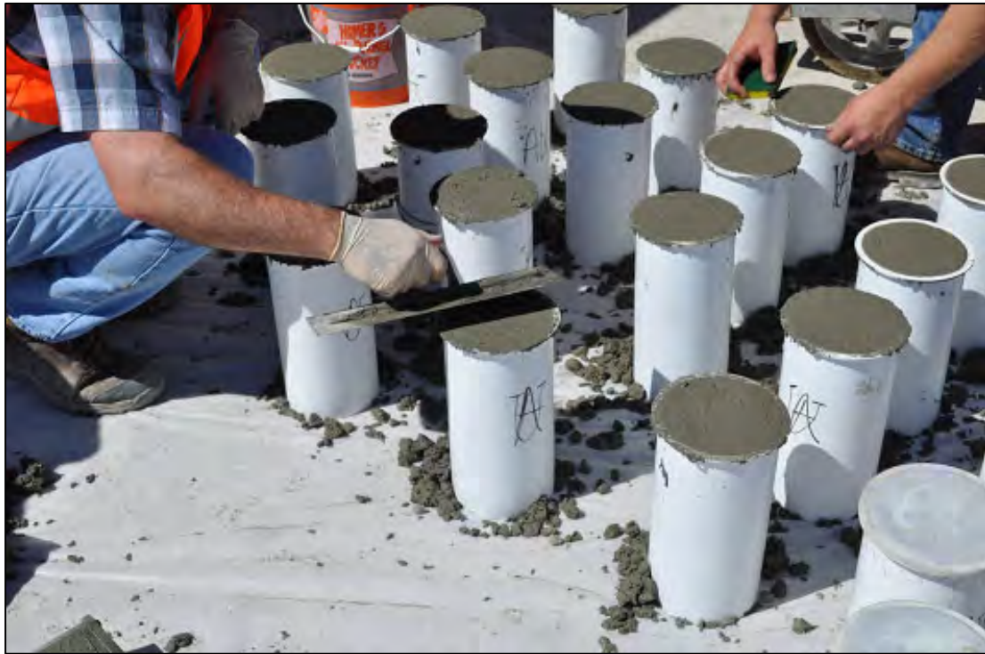
Figure 4-2: Preparation of concrete cylinders on the jobsite
