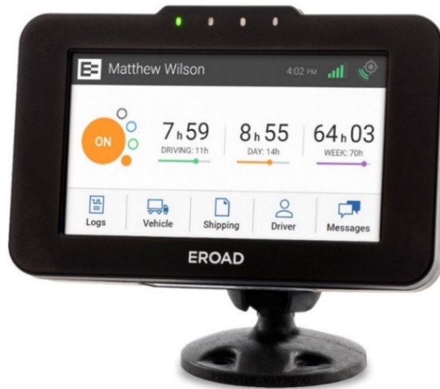
Figure 7. Illustration. In-vehicle device installed in trucks as part of the Eastern Transportation Coalition Phase 2 truck pilot.
