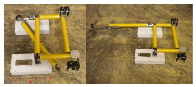
Figure 2. The final RABIT configuration is shown folded for transport (left) and with an extended outrigger (right). There is a wheel on the end of the outrigger and two wheels on the right side of the frame.
