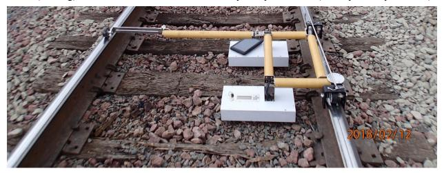
Figure 1. This photograph shows the RABIT deployed on an outdoor track with the antennas (the white boxes) straddling a tie and the frame resting on the track.
