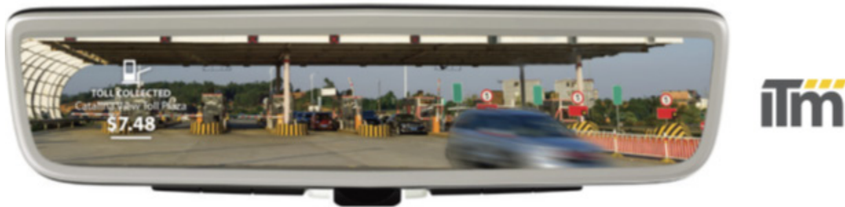
Figure 27. Photo. Gentex Integrated Toll Module® multiprotocol transponder built into a rearview mirror.
