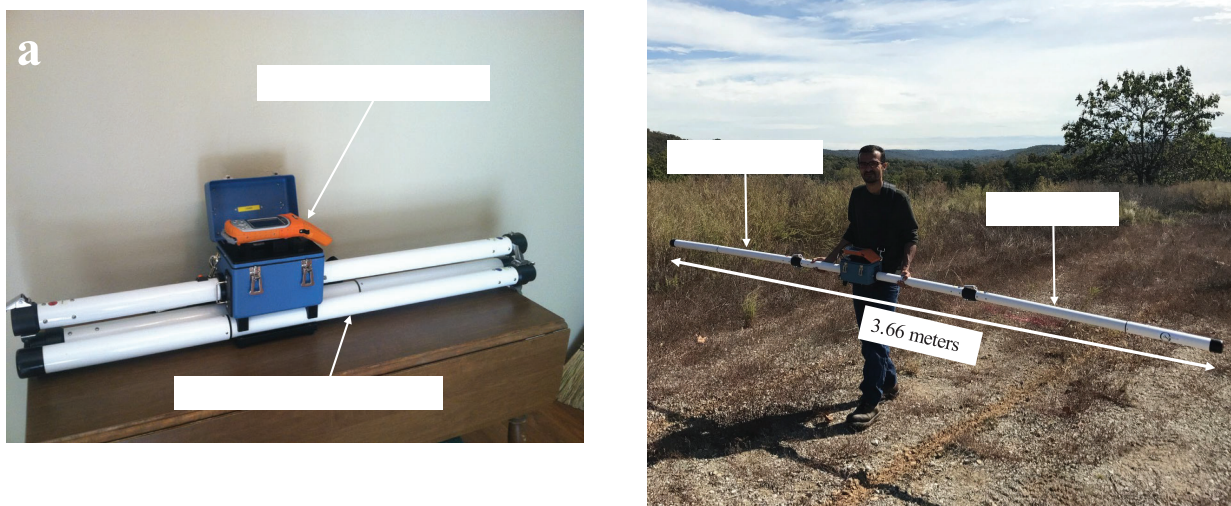
Figure 2.14- EM 31-Mk2 device. a) the main components of the EM31-MK2 device, b) field testing using EM31-MK2 device.
