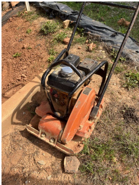
(a) plate compactor
