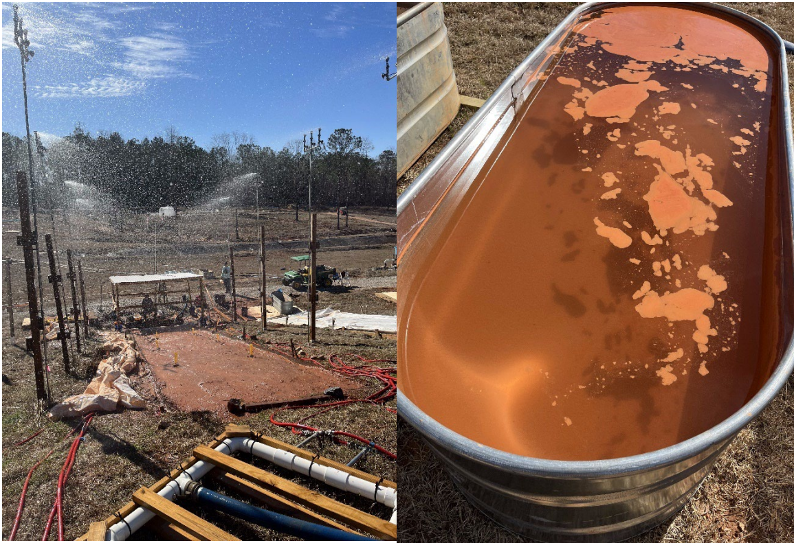
(a) rainfall simulator operation (b) filled runoff collection tank Figure 4-21: First Bare Soil Test on New ASTM D6459-19 Rainfall Simulators
