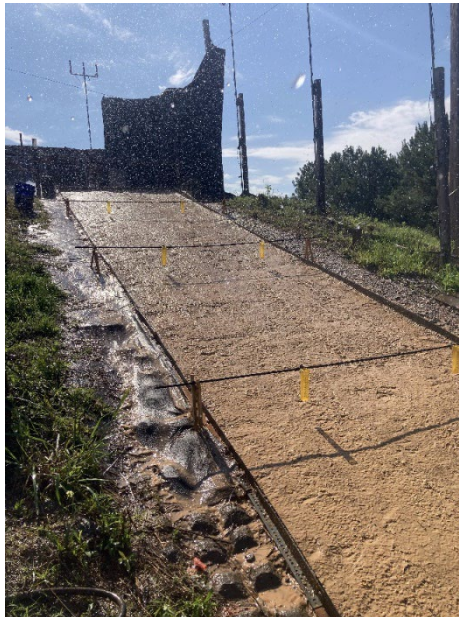
Figure 3-26: Rainfall Gauge Suspension Method
