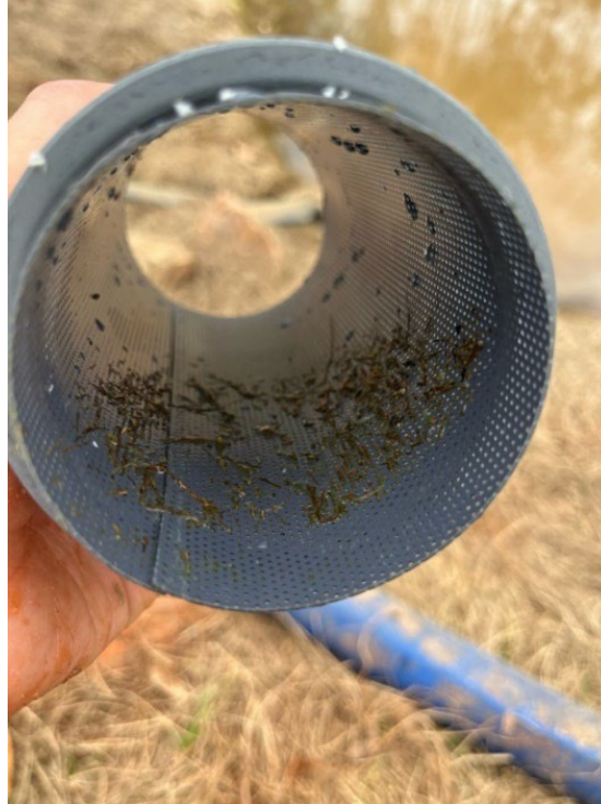
Figure 3-19: Debris Caught by Filter
