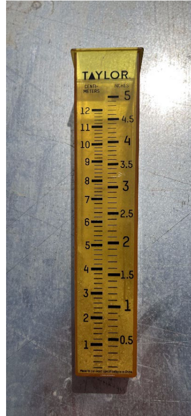
(b) Rainfall gauge
