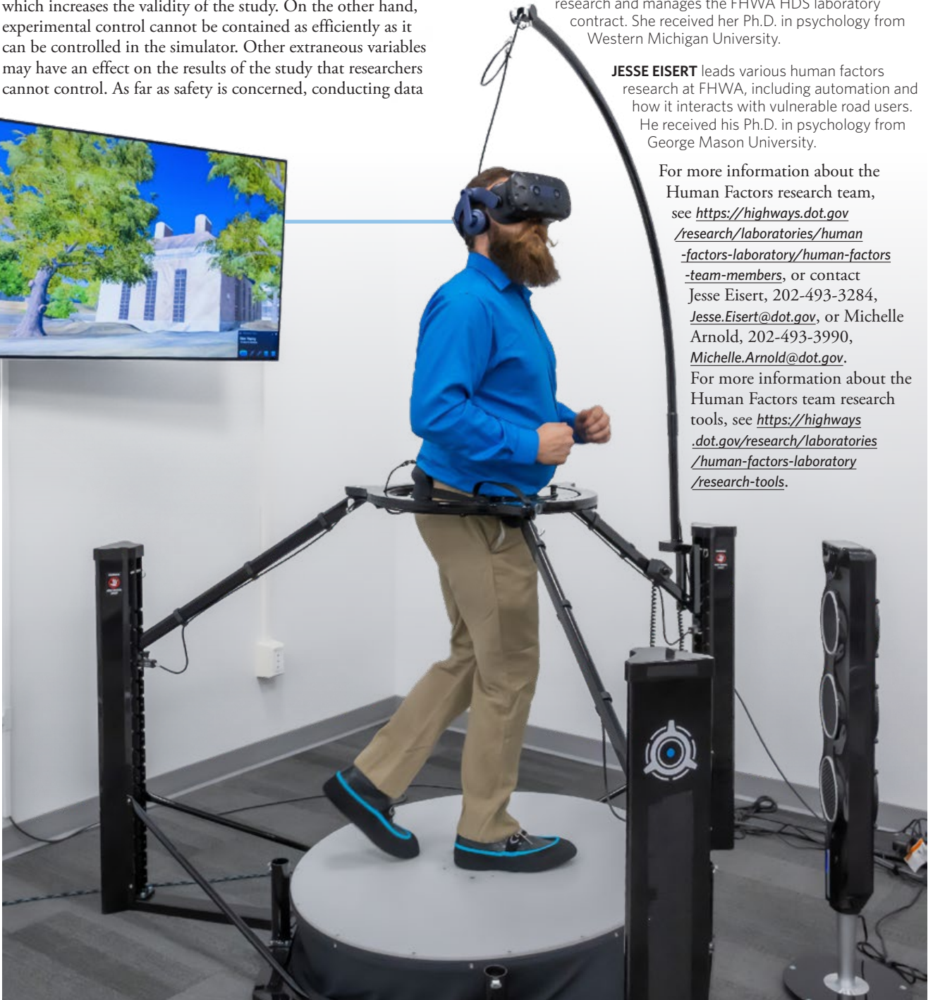
A member of the FHWA Human Factors team uses a virtual reality omni-directional treadmill.
