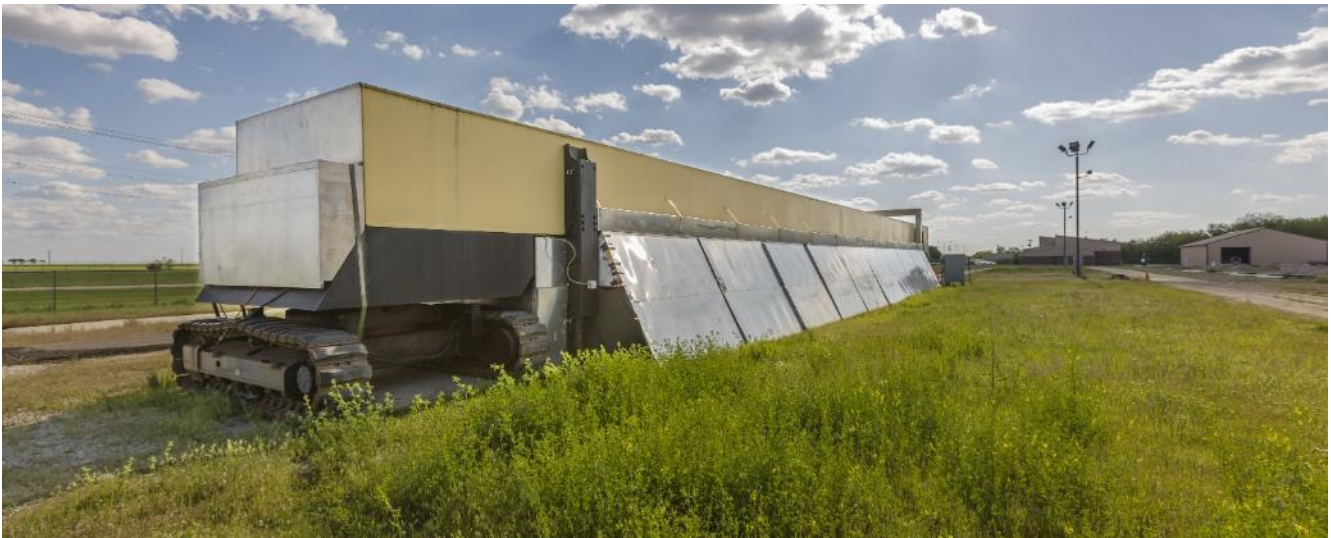
Figure 9. Photo. Temperature control panels as viewed from outside.
