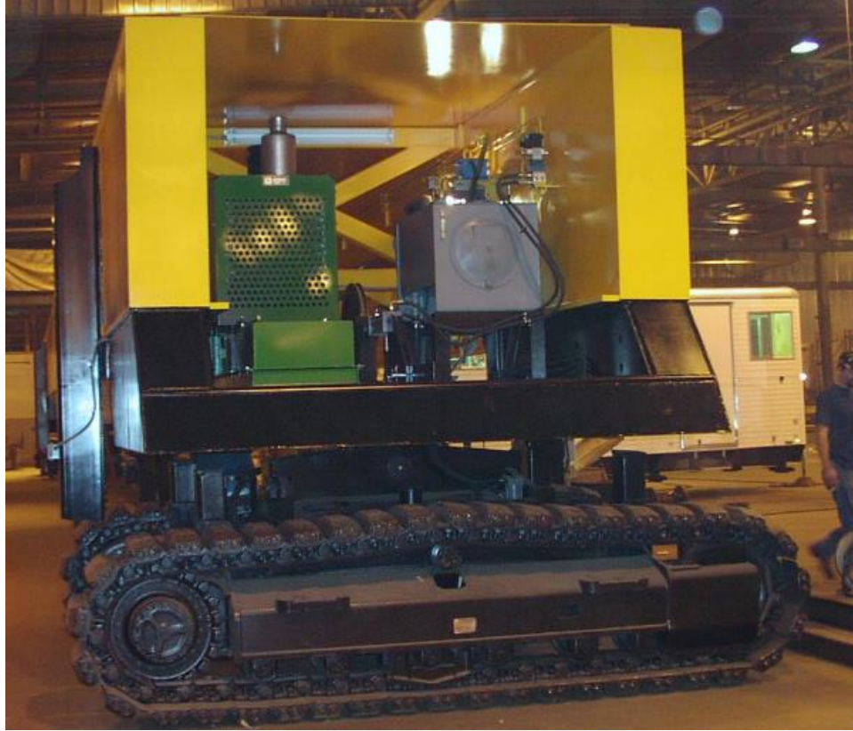
Figure 3. Photo. Diesel engine that operates the crawler track system.
