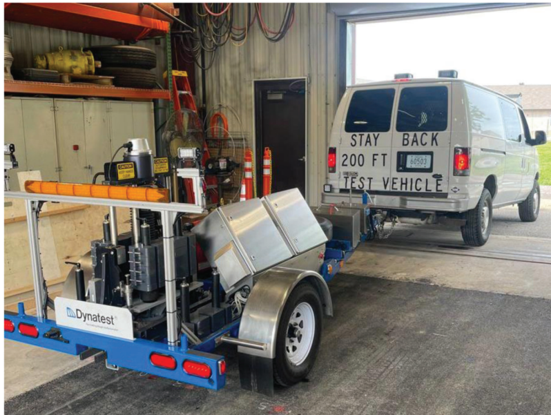
Figure 6.14 Falling weight deflectometer (FWD).
