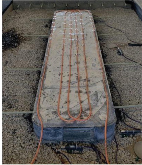
Figure 4.4 Magnetizable concrete DWPT unit in rigid pavement section.
