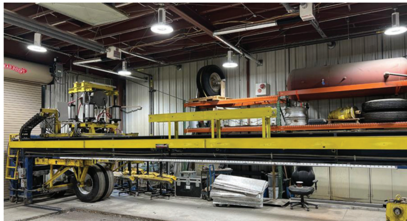
Figure 4.1 Accelerated pavement testing mechanism (vehicle prototype on steel frame carriage).
