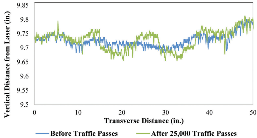
Figure 6.32 Transverse profile before and after 25,000 passes when the laser was placed in the middle of the flexible pavement (10 ft. away from longitudinal edges).
