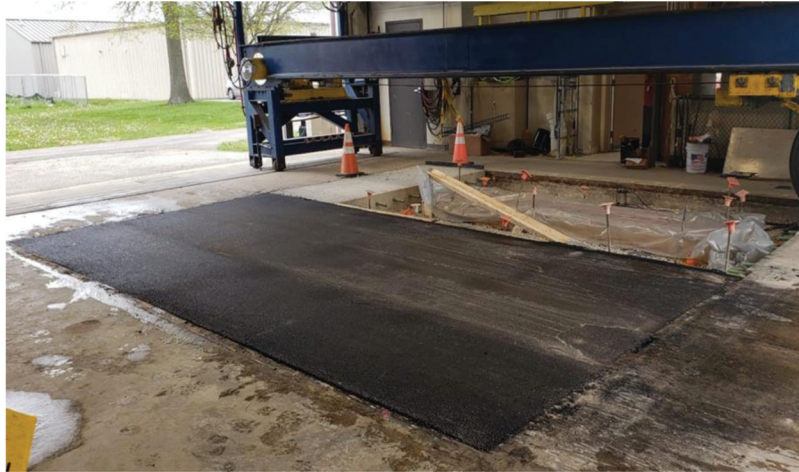
Figure 5.10 Flexible pavement section after construction.
