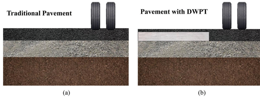
Figure 4.8 (a) Cross section of traditional pavement, and (b) cross-section of pavement with embedded DWPT.
