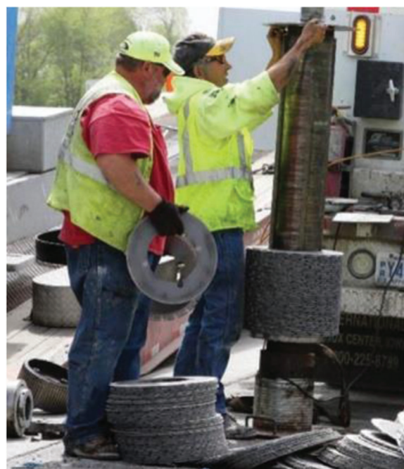
Stacking spacers and blades on a diamond grinding machine's cutting head (Smith et al., 2022).
