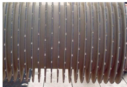
Diamond grooving cutting head (Smith et al., 2022).
