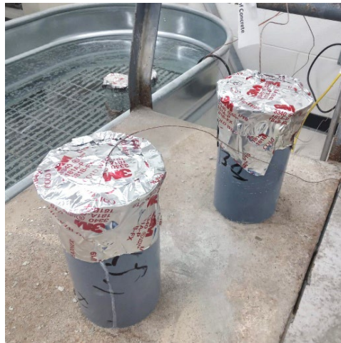
Figure 3-4 Maturity cylinders with embedded sensors during initial curing.
