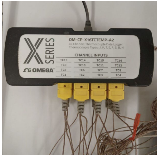
Figure 3-5 A 16-channel data logger for monitoring of 8 different concrete mixes.
