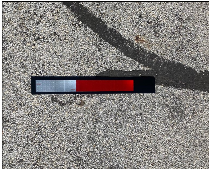
Figure B-3. Reflective Tape that Triggers AMES Profiler
