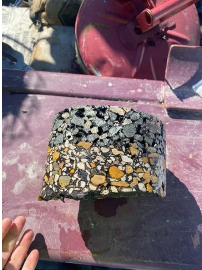
Figure 58. Core from US 69 showing PFC bonded to underlying HMA.
