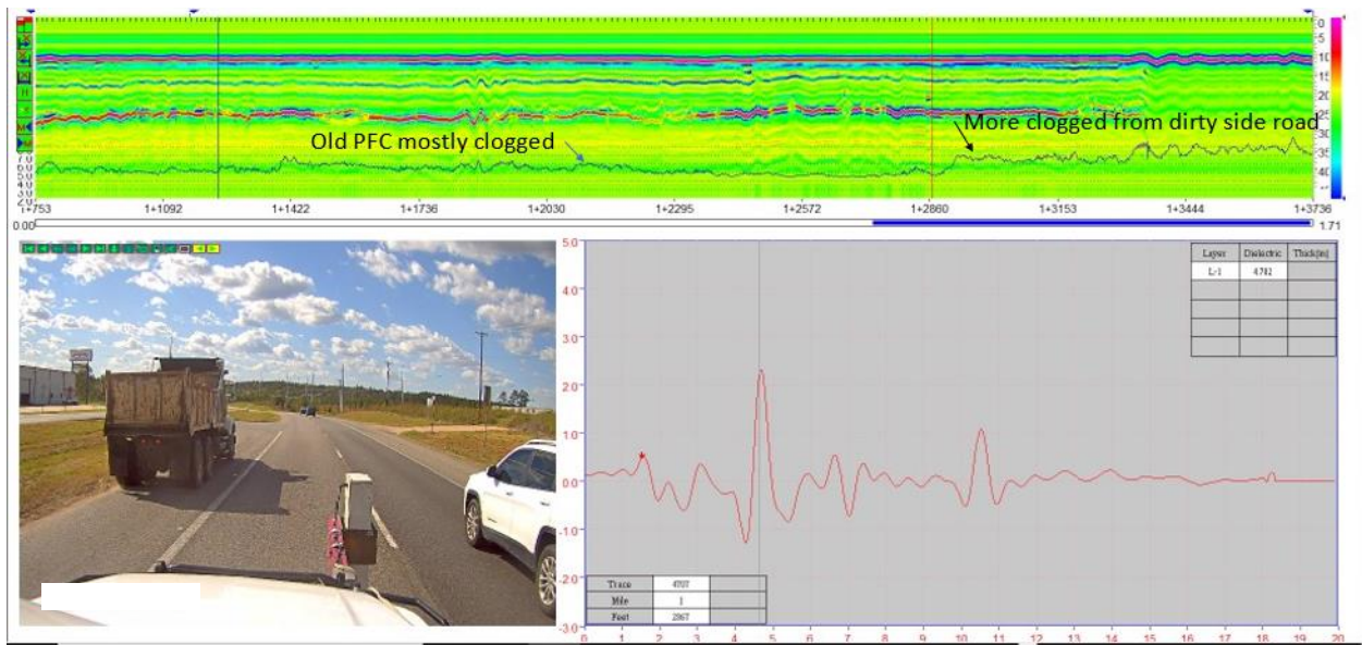
Figure 53. GPR data for left lane of US 69.
