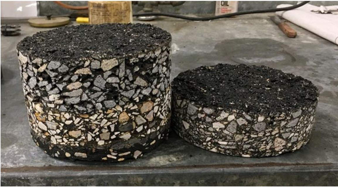
Figure 106. Photo of core after shear test.
