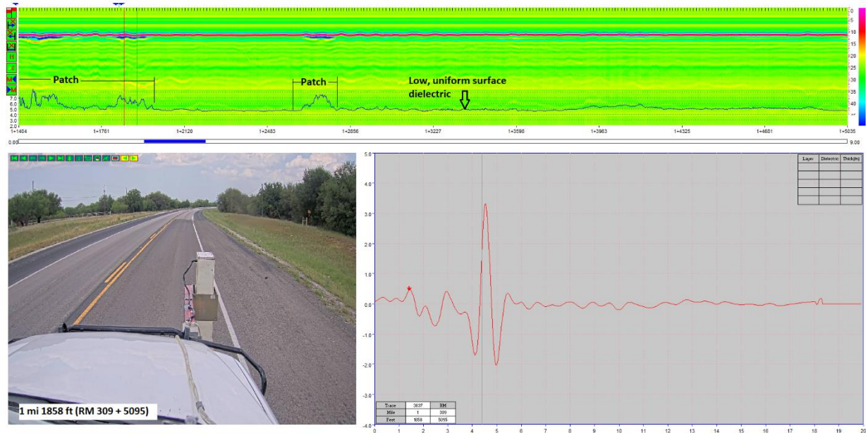
Figure 69. GPR data on US 183 south of Breckenridge.
