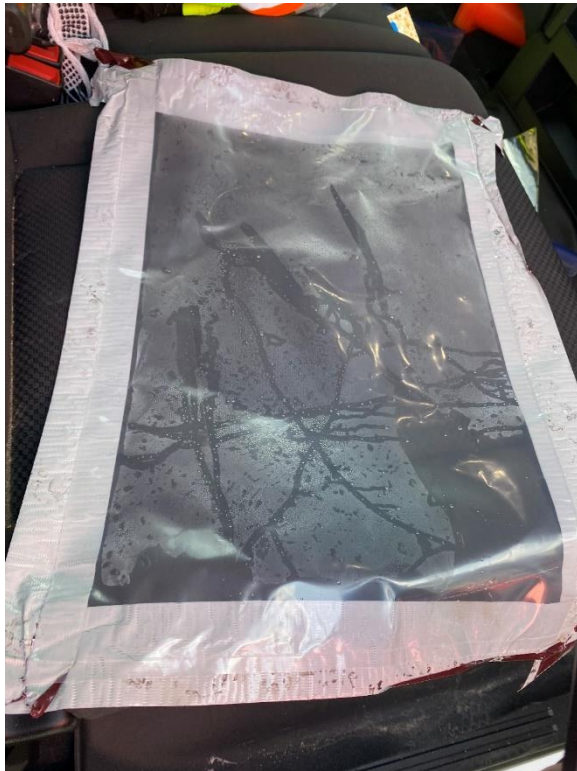
Figure 96. Plastic sheeting after removal from pavement surface after 10 minutes.
