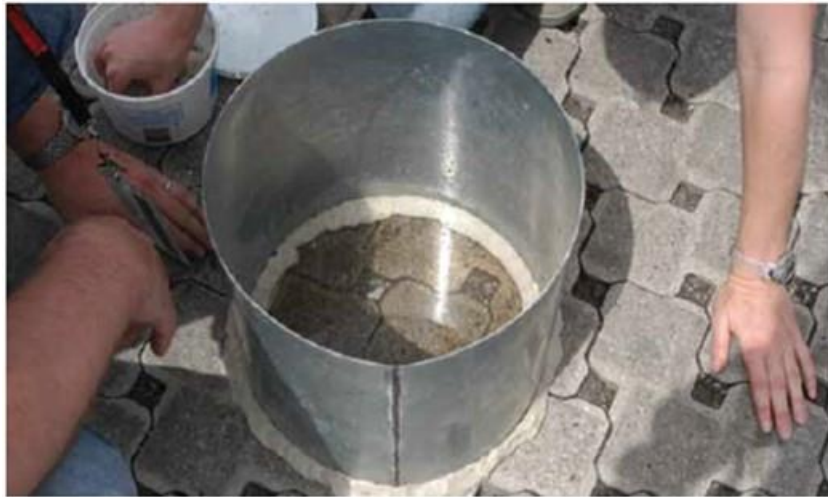
Figure 24. Single-ring infiltrometer used to measure water infiltration rate on permeable pavements (Kinter 2010).
