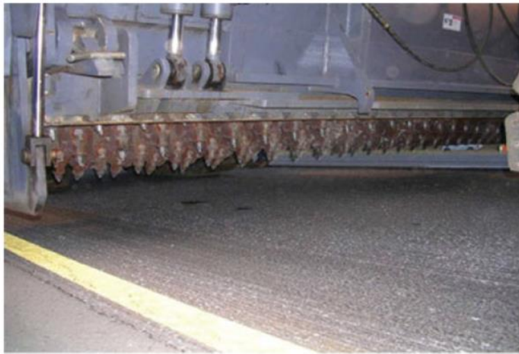
Figure 18. Micromilling equipment teeth (Jared and Hines 2014).
