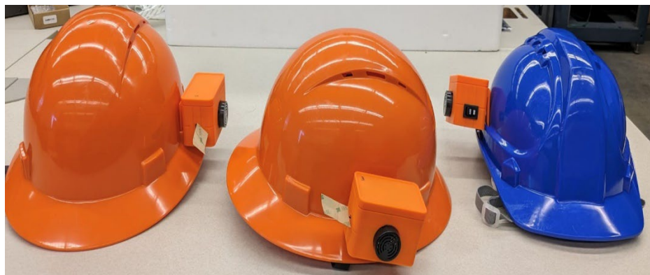
Figure 3.7 Wearable Proximity Sensor (WPS) Tags Attached to Safety Helmets
