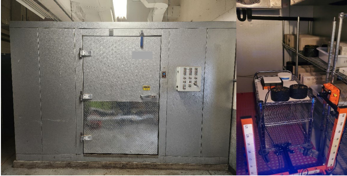
Figure 1. Photo. Temperature-controlled environmental chamber accommodates HMA specimens and the DPS (FHWA 2024).
