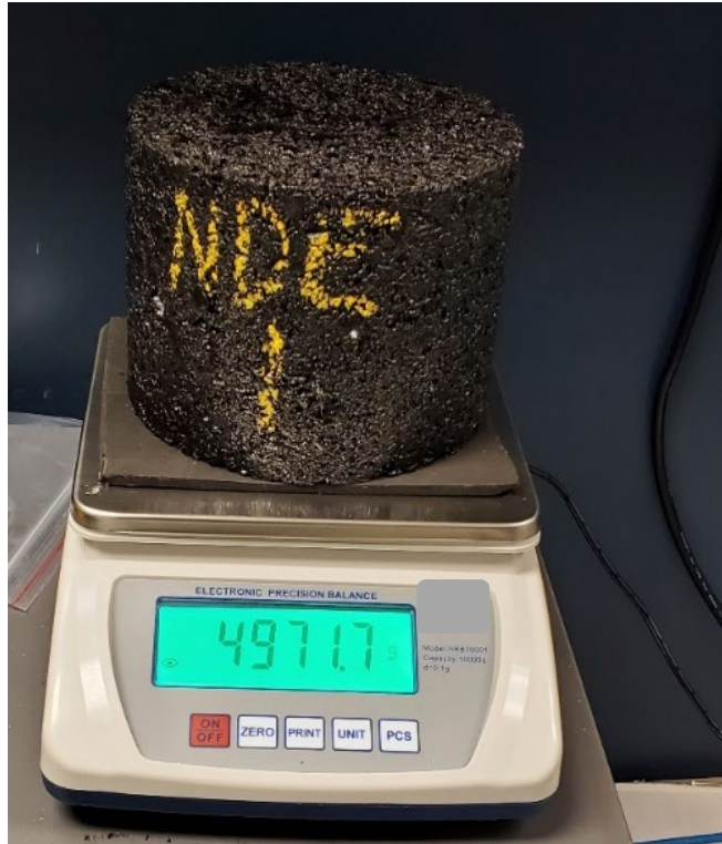
Figure 6. Photo. Measuring the amount of sprayed water on the SGC sample.
