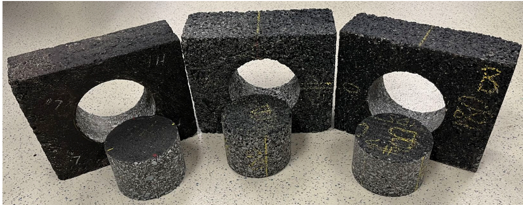
Figure 41. Photo. Fabricated HMA slabs with cores drilled from center of corresponding slab.
