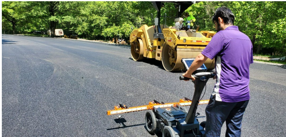
Figure 53. Photo. An NDE laboratory research engineer performing DPS scanning.
