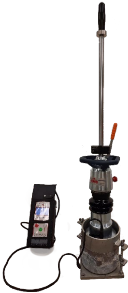
Figure 1 LWD test on Proctor mold.
