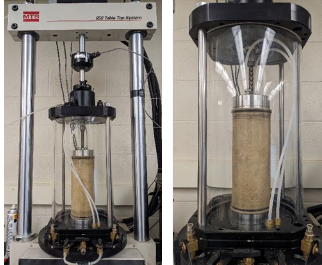
Figure 2-14 MTS 858 load frame (left) and 4-in specimen cells (right) for RLTT.
