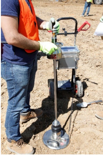
Figure 2 LWD test in the field.
