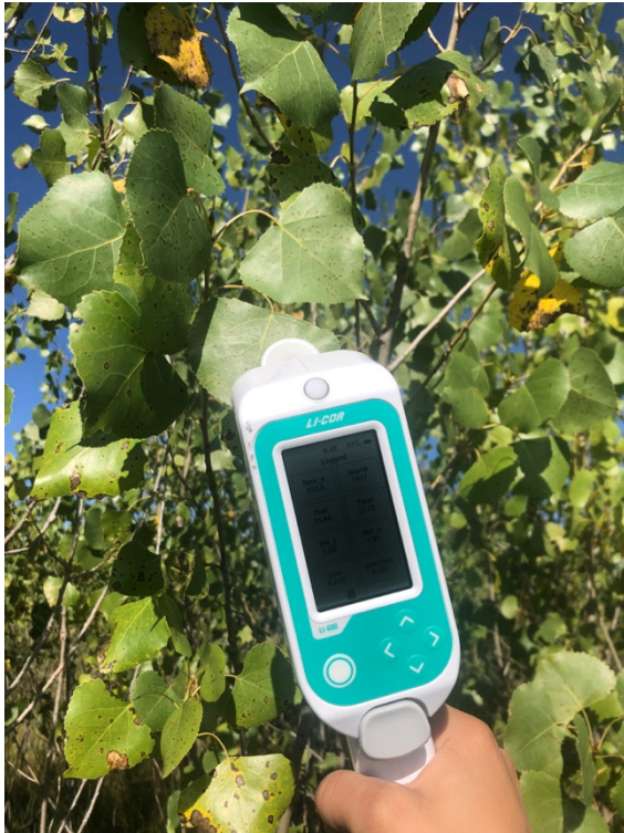
Figure 4: Measuring stomatal conductance with the LI-600 (LICOR Environment, Lincoln, USA) on a P. deltoides leaf. The handheld instrument simultaneously records leaf and air vapor pressure deficit, leaf and air temperature, and solar radiation.
