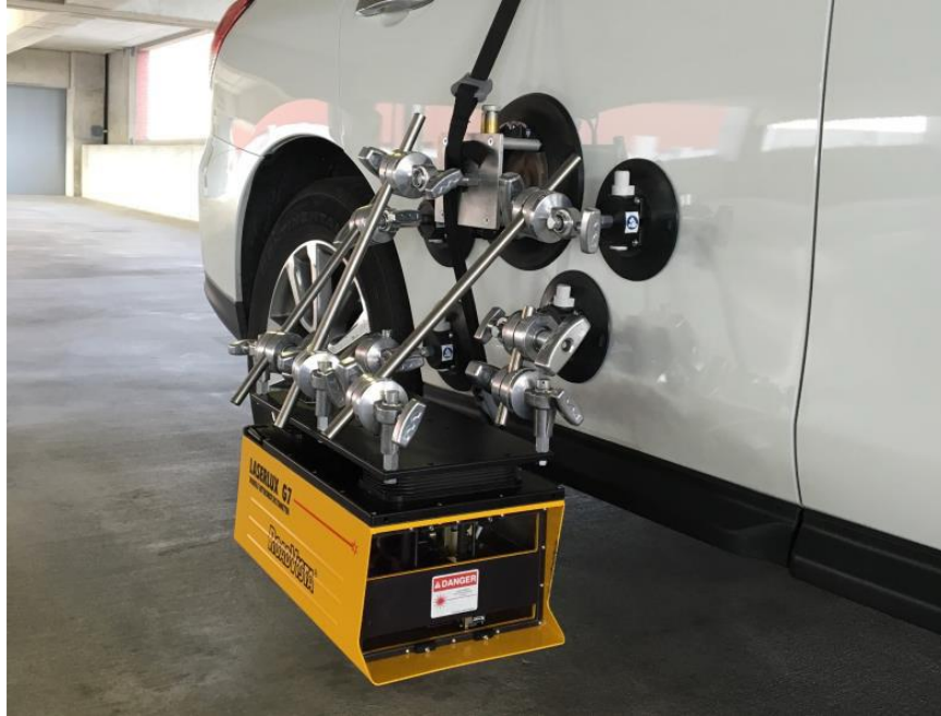
Figure 3-3: LLG7 Mounted to a Vehicle using the Squid Mount™ (Austin & Schultz, 2020).
