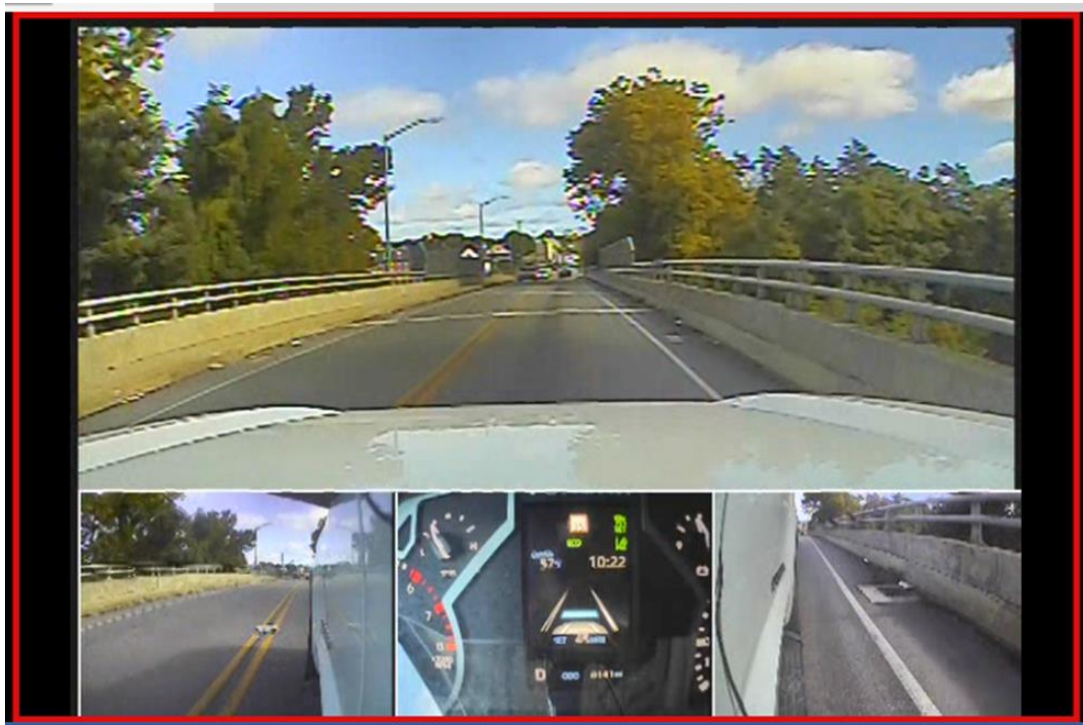
Figure 5-16: Failure to Detect Lane Markings Due to Object on the Marking.
