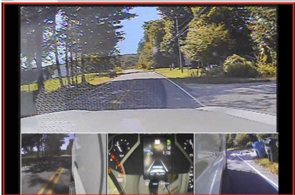
Figure 4-27: Screen Capture of ADAS Operating with Interruptions.
