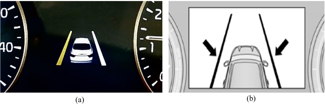
Figure 4-3: A Qualitative Layout of Lane Marking Detection-Related Visual Cue; (a) Only Left Lane Detected, (b) Both Lanes Detected (Jeep Grand Cherokee, 2022).
