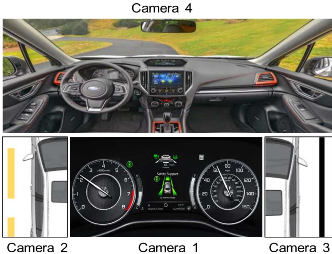
Figure 4-18: VBOX Camera Setup Layout for Data Collection (MotorTrend, 2023).
