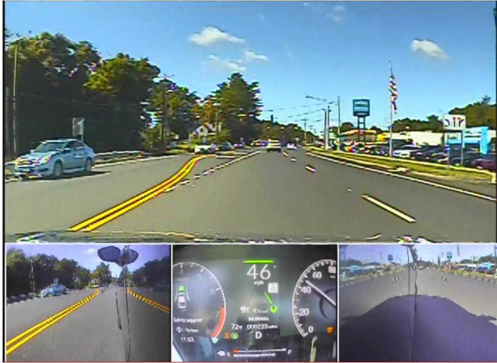
Figure 5-13: Failure to Detect Lane Marking with Changes in Marking Type and Color.
