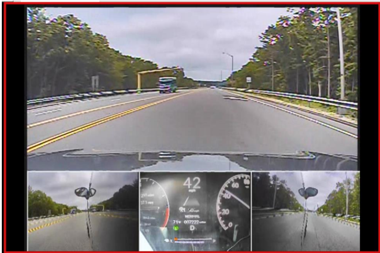
Figure 5-17: Failure to Detect Lane Marking in Wide Lane.
