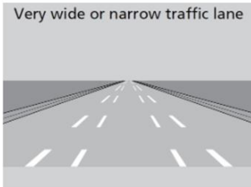
Figure 4-15: Detection Issue with Very Narrow or Wide Lane Markings (Honda, 2022).
