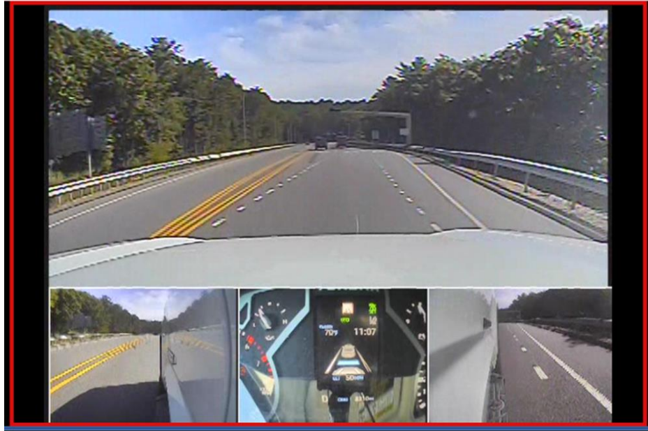
Figure 5-15: Failure to Detect Lane Marking with Changes in Marking Type.
