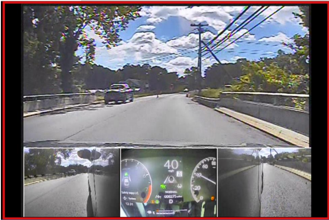
Figure 5-18: Detected Pavement Joint as Lane Marking.
