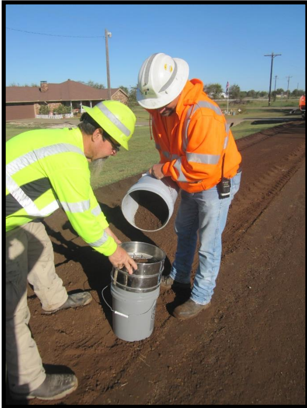
100% passing 1¾-in. sieve. 85% (min.) passing ¾-in. sieve
