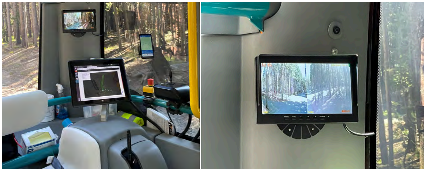
Figure 18: Additional Monitor Added to Address Blind Spots
