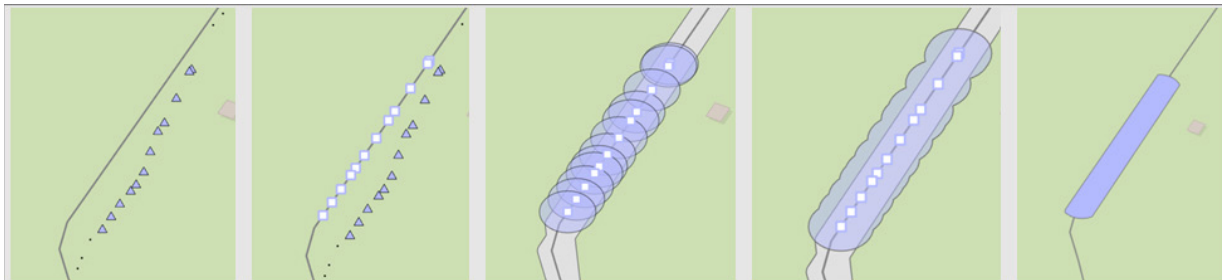
Figure 6: Five-step process for creating spatial polygons from target pings for designated segments.
