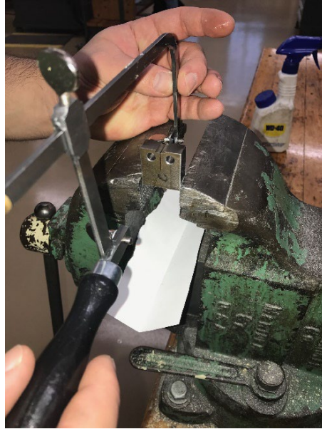
Figure 46. Cutting sharp notch at the base of waterjet cut notch using jeweler's saw
