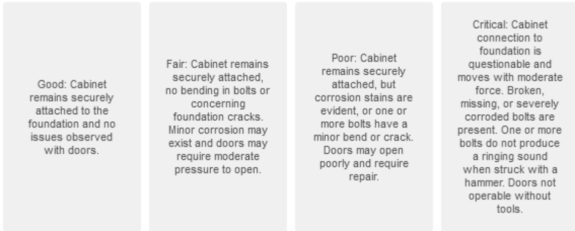
Figure 46. Illustration. Condition levels for traffic signal cabinet anchoring.
