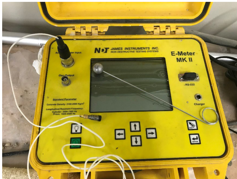
Figure 4.3: James E-Meter Mk II with Accelerometer and Impactor
