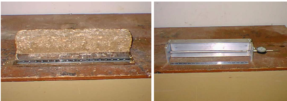
Figure 2.8: Test Sample and Setup for Shrinkage Testing
