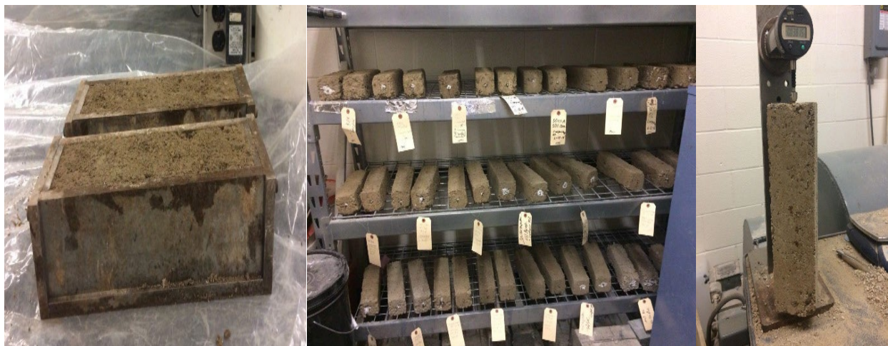
Figure 3.7: Shrinkage Test Setup, Curing, and Length Measurement
