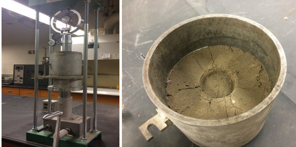
Figure 3.8: CBR Test Setup and a Tested Specimen
