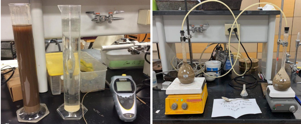
Figure 3.3: Hydrometer and Specific Gravity Test on Clay
