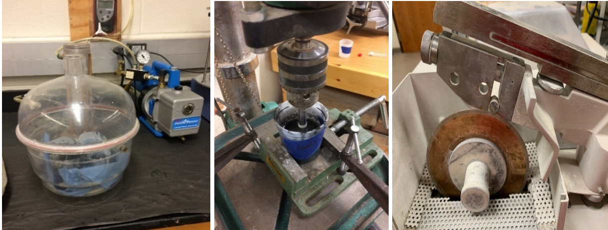
Figure 3.12: SEM Sample Preparation, Epoxy Curing, and Sample Coring and Cutting
