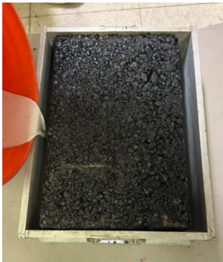
d) Plaster applied on the sides
