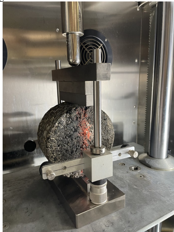
Figure 4.9: IDT test setup.
