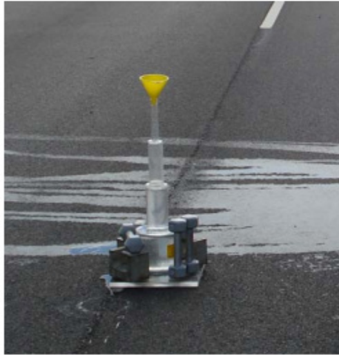
Figure 2.7: NCAT Permeameter. (Stephen and Sushanta 2009)
