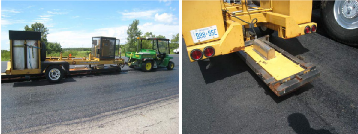
Figure 2.12: Infrared joint heater by Head Design Equipment, Inc. (Williams 2011)
