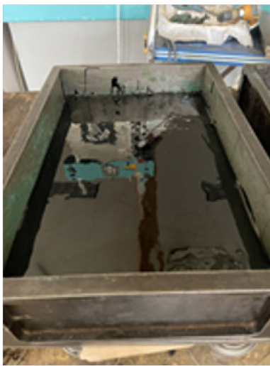
c) Base pavement slab after application of emulsion
