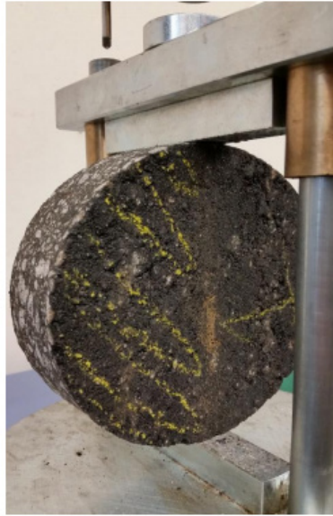
Figure 2.8: Indirect tensile strength. (Kim 2017)
