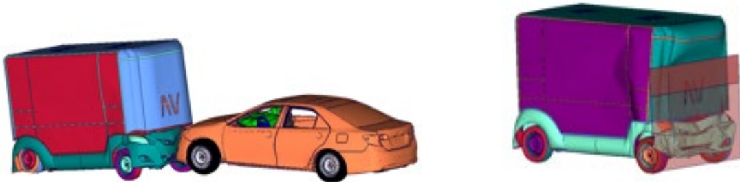
Figure 17. (a) 40.2 km/h (25 mph) sedan into ADS 1 shuttle; (b) ADS 1 shuttle 40.2 km/h (25 mph) rigid wall impact after 100 ms
