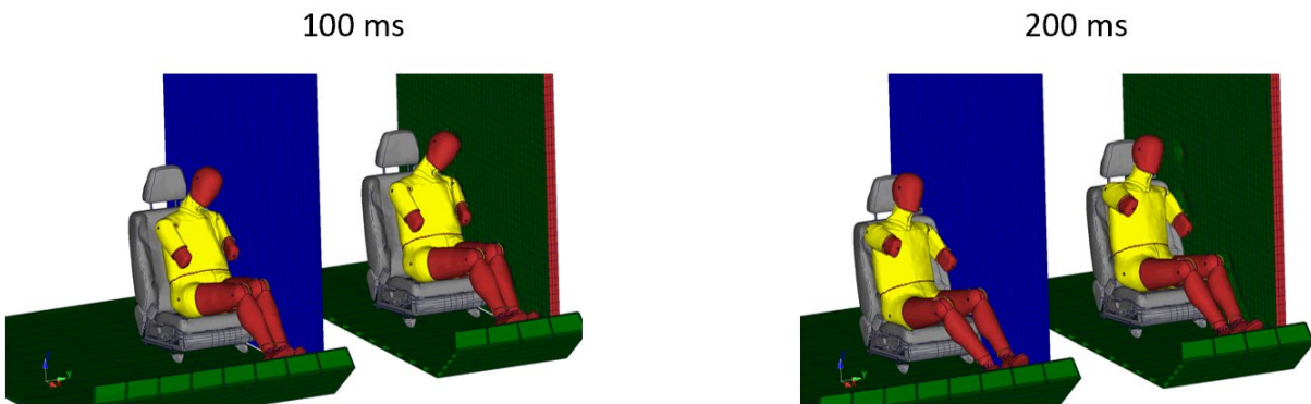
Figure 49. Side impact kinematics unbelted next to non-deformable and “201-compliant” surfaces after (a) 100 ms; (b) 200 ms
