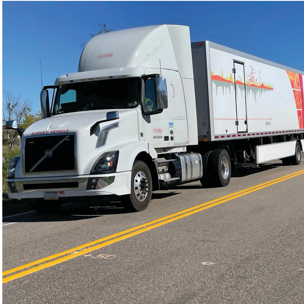
© Gerardo Flintsch, Virginia Tech Transportation Institute. TSDDs being used on a highway.
