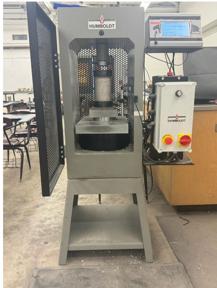
Figure 2: Humboldt HCM-500-iHA Compression Tester of the California State University Long Beach
