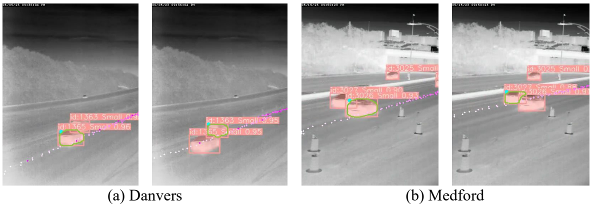
Figure 3.8. Tracking of occluded and occluding vehicles
