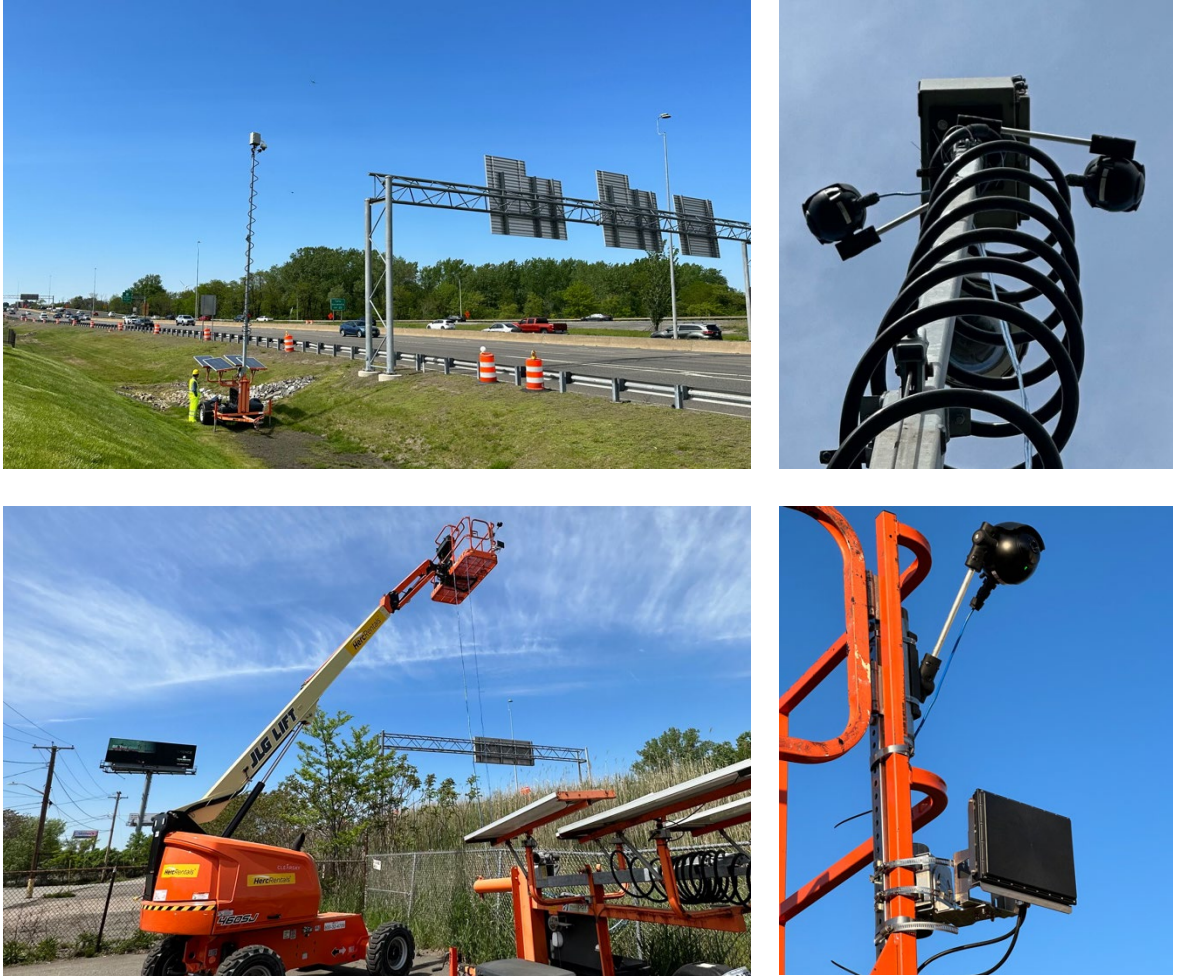
Figure 2.5. Thermal cameras and radar systems at Medford
