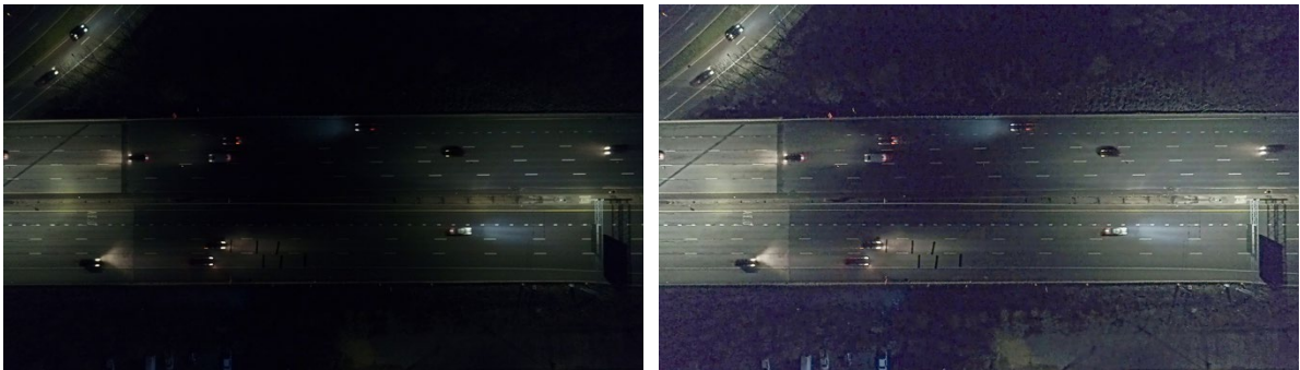
Figure 3.12. Nighttime image before and after applying enhancement
