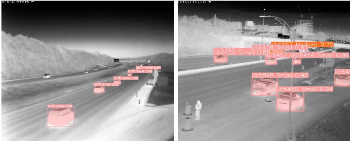
Figure 3.5. Vehicle segmentation output generated by the YOLOv8 large model
