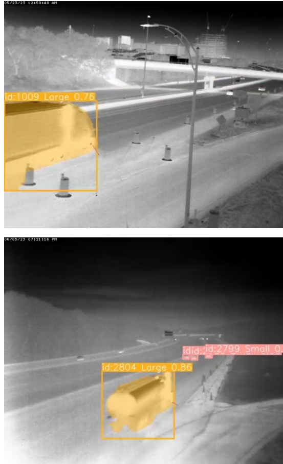
Figure 3.9. Vehicles traveling too close to work zone lane closure taper
