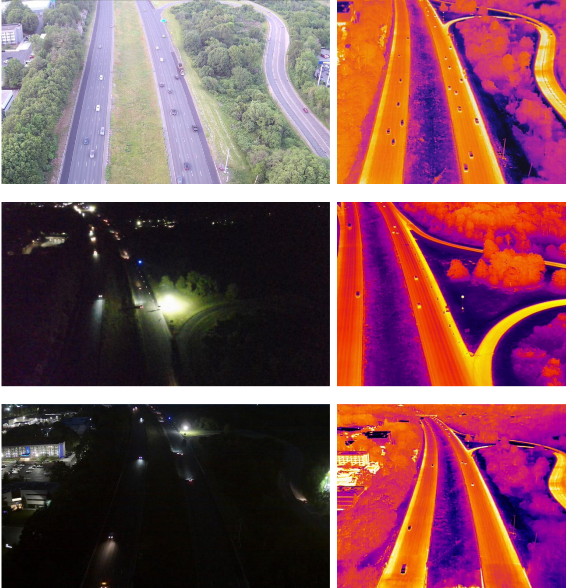
Figure 8.42. RGB versus thermal drone footage under varying light conditions in Danvers
