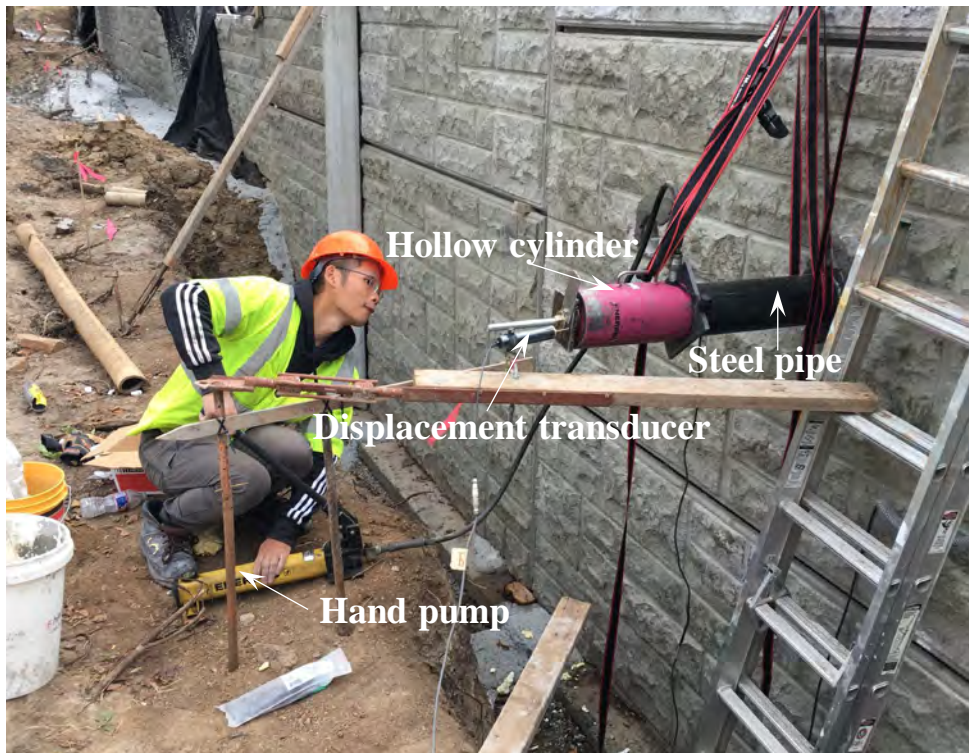
(b) Pullout Test Setup in Field
