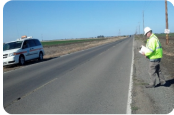
Figure 10. APCS Vehicle on the Road and Manual Pavement Inspection
