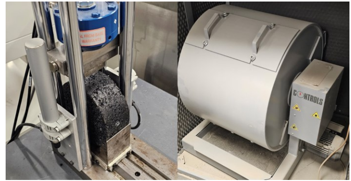
Figure 1. Two Performance Tests for HMCL Mixes (Left: Ideal Rutting Test; Right: Cantabro test).
