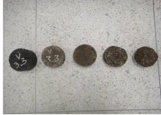
(b) Increasing Cantabro Loss as Flux Oil Content Decreases
