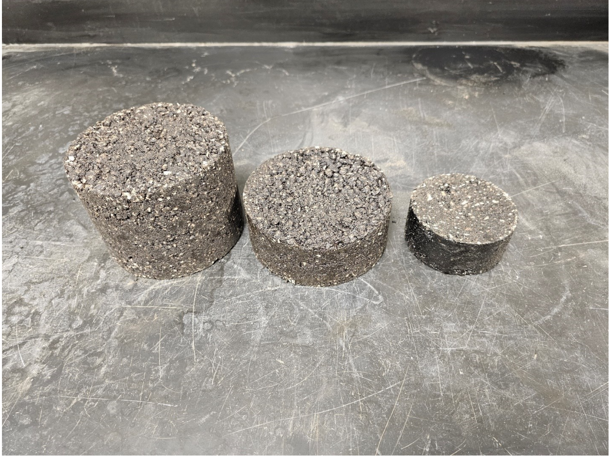
Figure 16. SGC (left), IDEAL-CT (middle), and TGC (right) Specimens.
