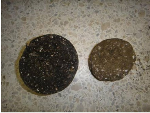
(a) LRA Specimen Before and After Cantabro Test
