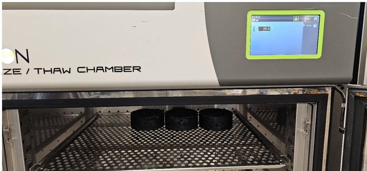
Figure 20. Conditioning of IDEAL-RT Specimens.
