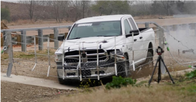
Figure 2. Full-Scale Crash Test with MASH Pickup Truck.
