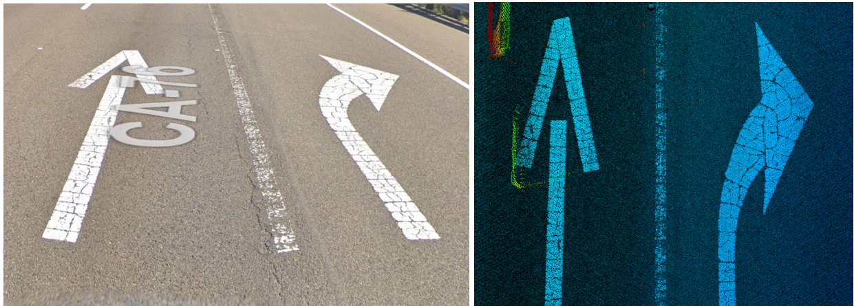
Figure 4. Example of the Road Condition on Road Marks in the Google Street Map (Left) and MTLs Point Cloud Data
