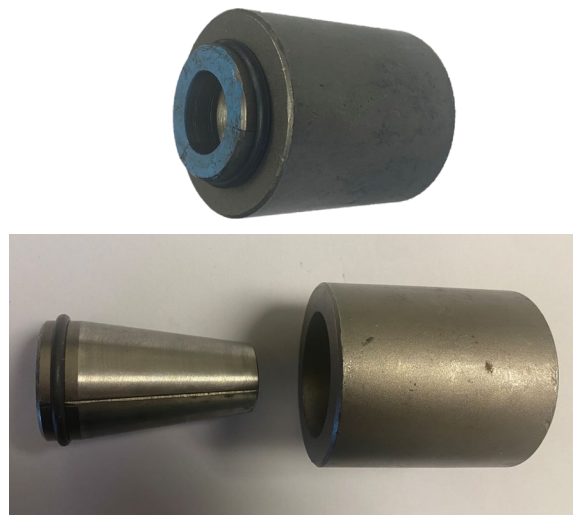
(b) Chuck without cap and spring (used at dead end)
