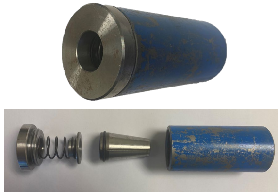
(a) Chuck with cap and spring (used at live end)
