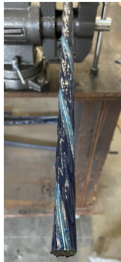
(c) Epoxy coating removed
