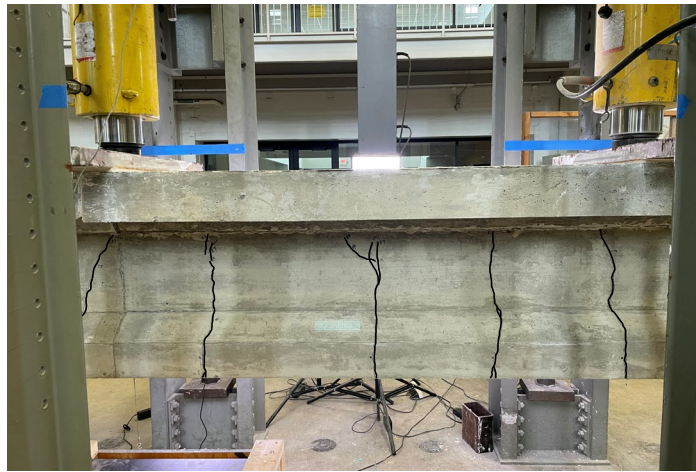
(b) Beam under load ( \Delta = 1.25 in. [31.8 mm], P = 101 kip [449 kN])
