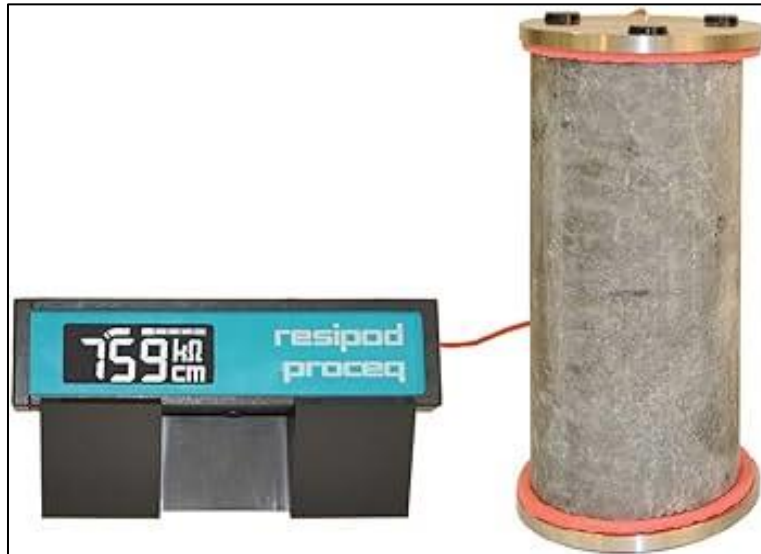
Figure 7-3: BR Measurement Using Resipod by Proceeq
