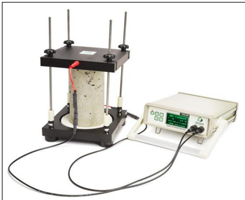
Figure 7-2: BR Measurement Using RCON by Giatech Scientific
