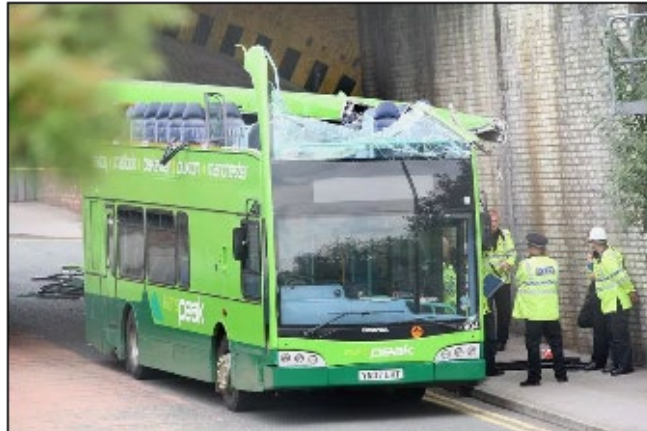
(a) A double-decker bus hitting a bridge in Manchester, UK. As a country widely adopting double-decker buses, the UK faces unique challenges of bridge/tunnel strikes.
