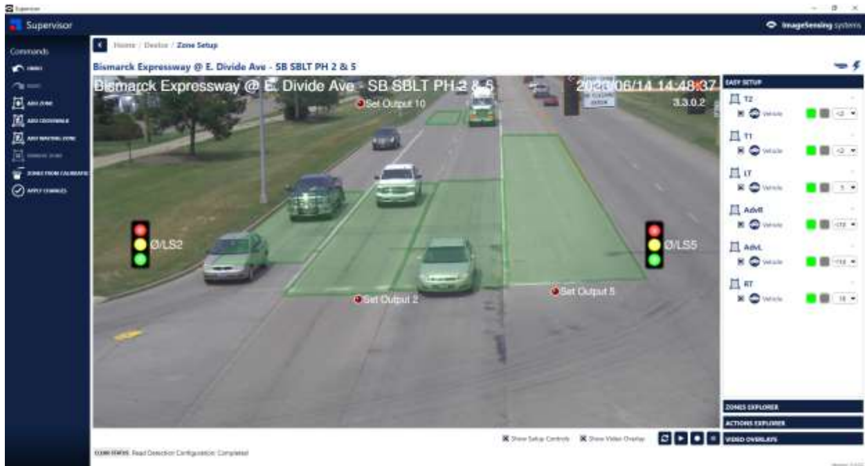
Figure 4. Updated setup with corrected zone labels and added zone
