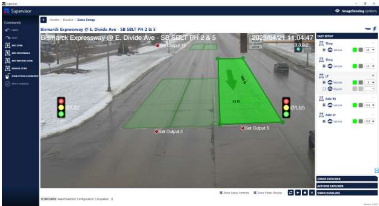
Figure 3. Non-conventional zone labels and missing (right-turn) zone
