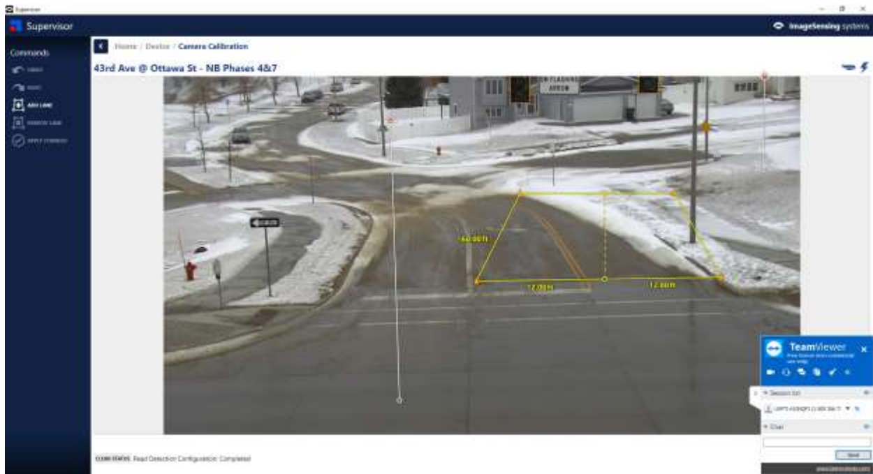
Figure 1. Sample existing camera calibration
