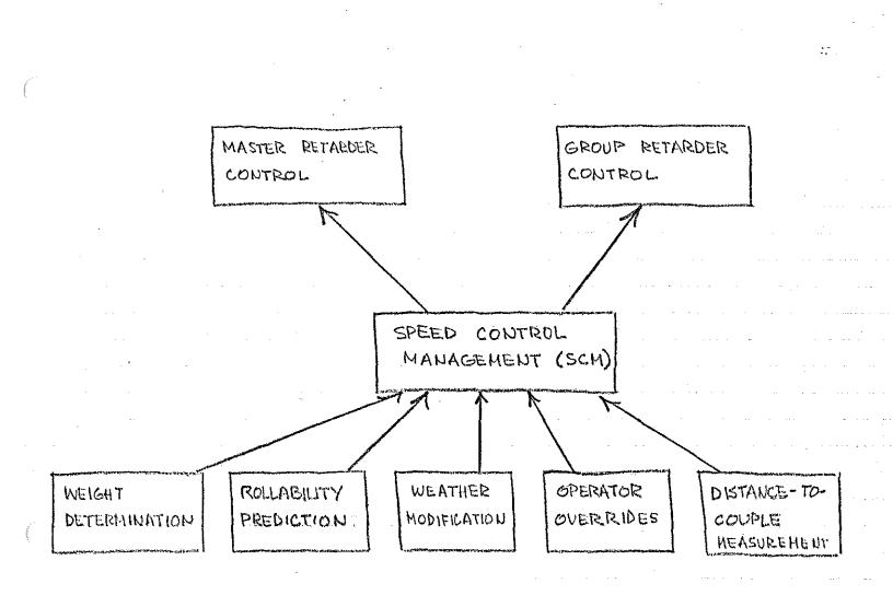
FIGURE 1: BLOCK DIAGRAM MAJOR FUNCTIONS
