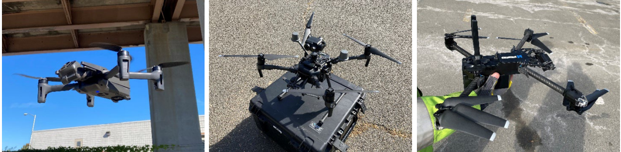
Figure 9 - Field-Tested Drones - Parrot Anafi USA, DJI Matrice 210, and Skydio X2 from left to right
