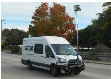
Figure 5 - Van Equipped with IR Sensor
