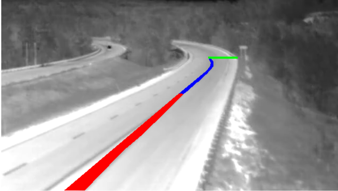
Figure 4-21. Merging region classification for merging point analysis at Littleton South.
