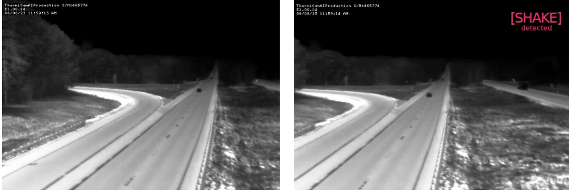
(a) Normal camera view. (b) Camera view change detected. Figure 4-11. Camera view change detection at Tilton North.
