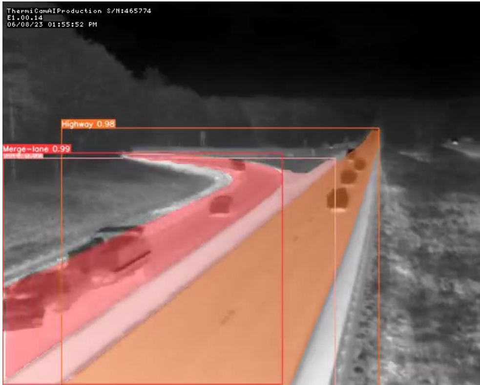
Figure 4-13. Segmentation mask illustrating detected roadway, gore, and merging lane areas.
