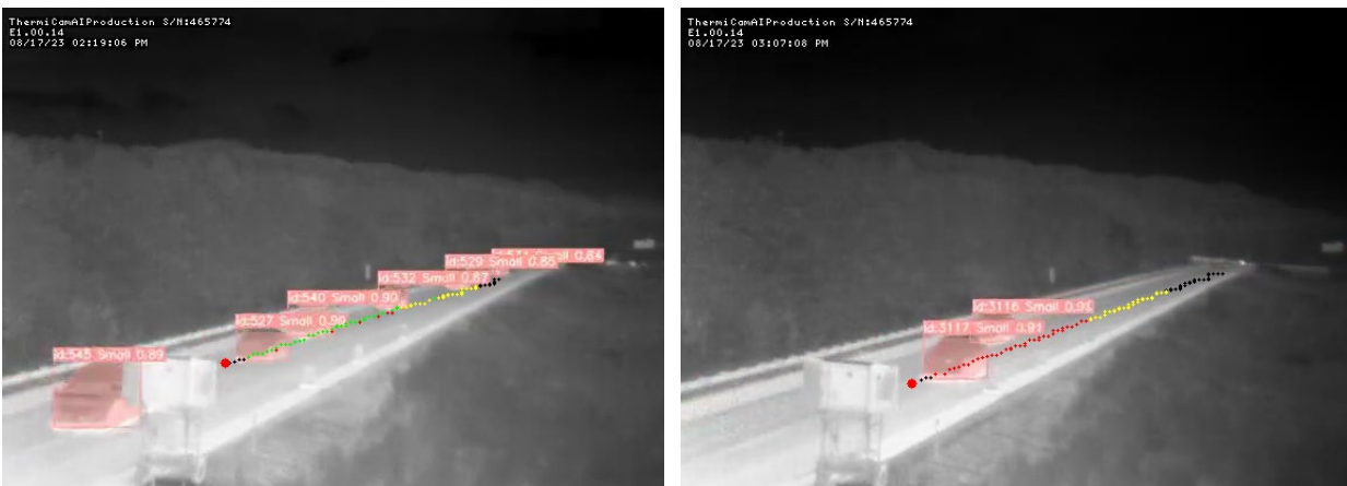
Figure 5-4. Samples of trajectory analysis showing vehicles merging in different regions.
