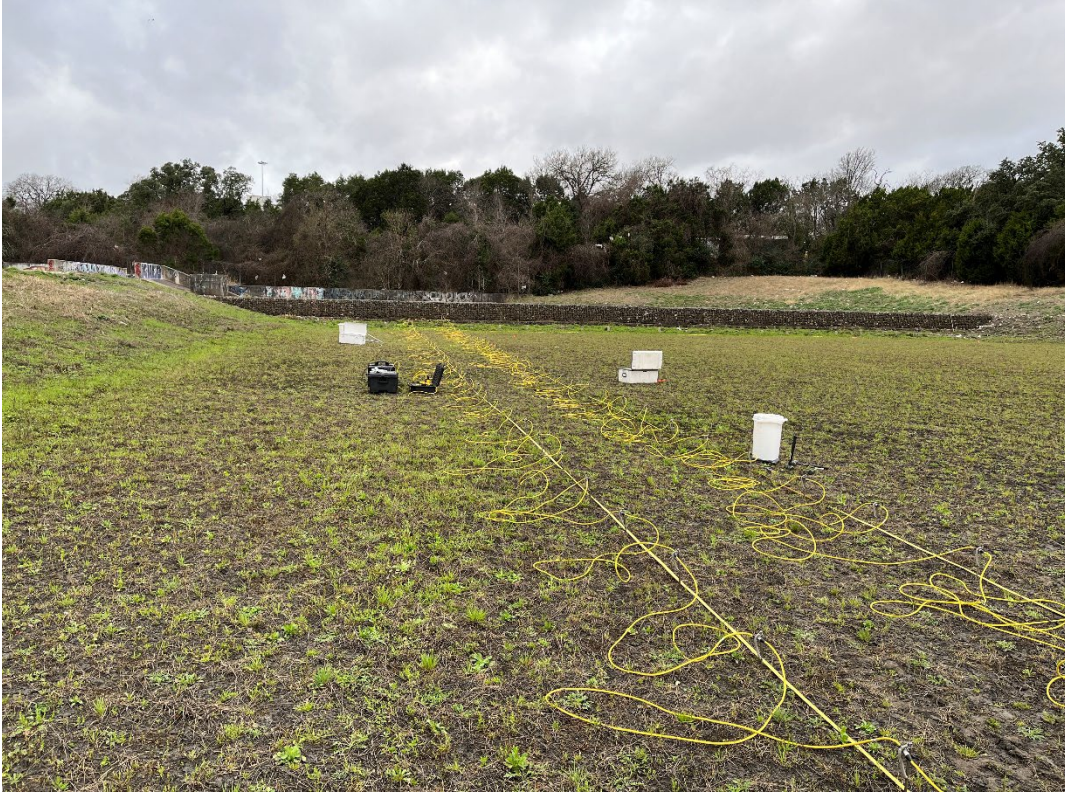
Figure 4.44: Testing on ERT line A, while ERT line B is in preparation.
