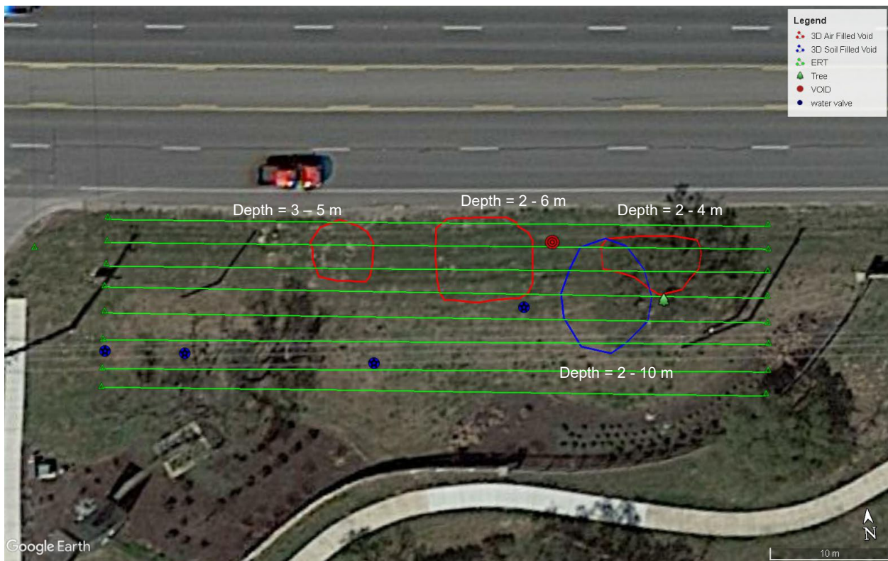
Figure 4.21: Surface map of suspected void locations based on the pseudo-3D ERT analysis.
