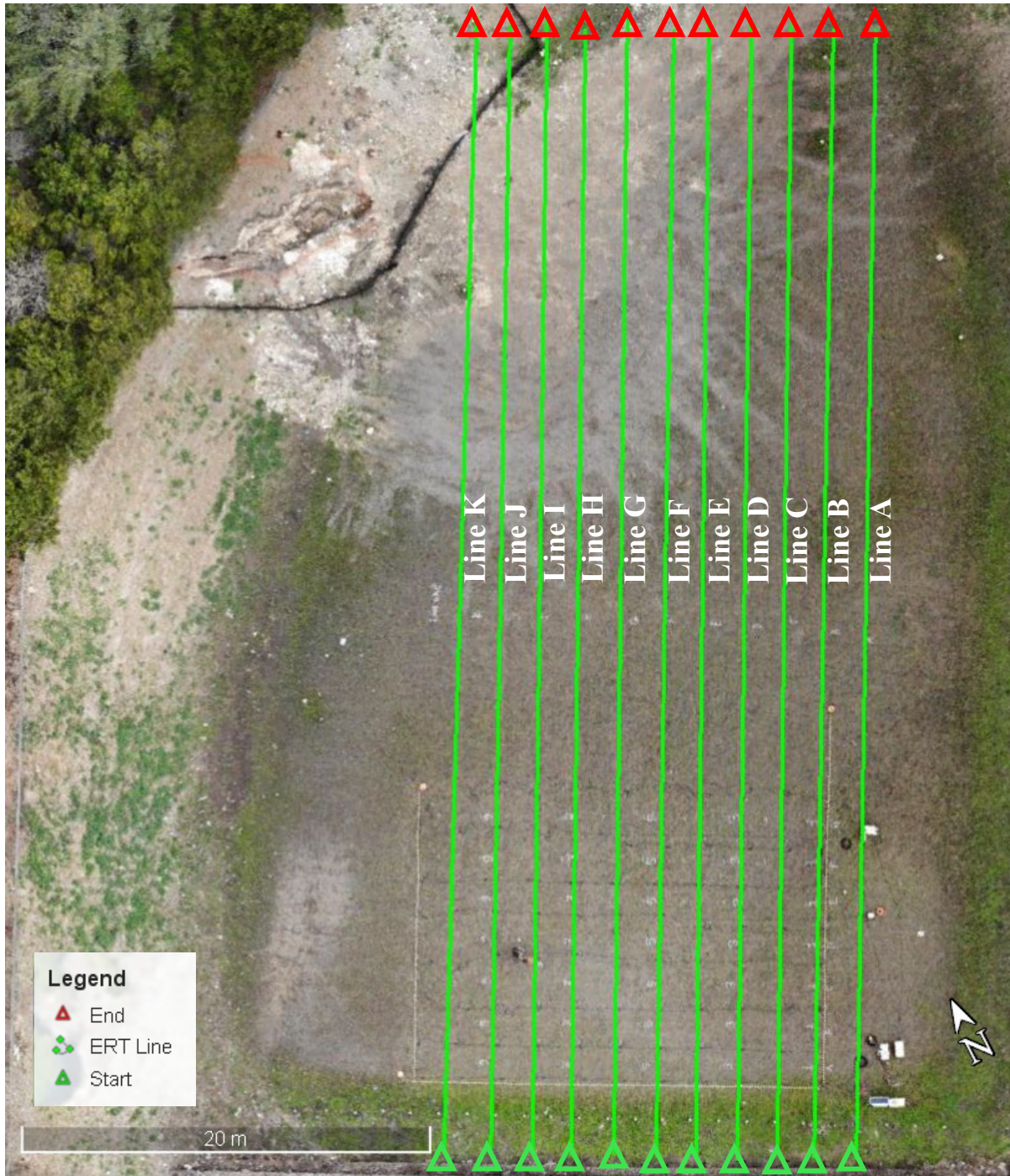
Figure 4.39: Site map of ERT testing showing the location of each ERT line.
