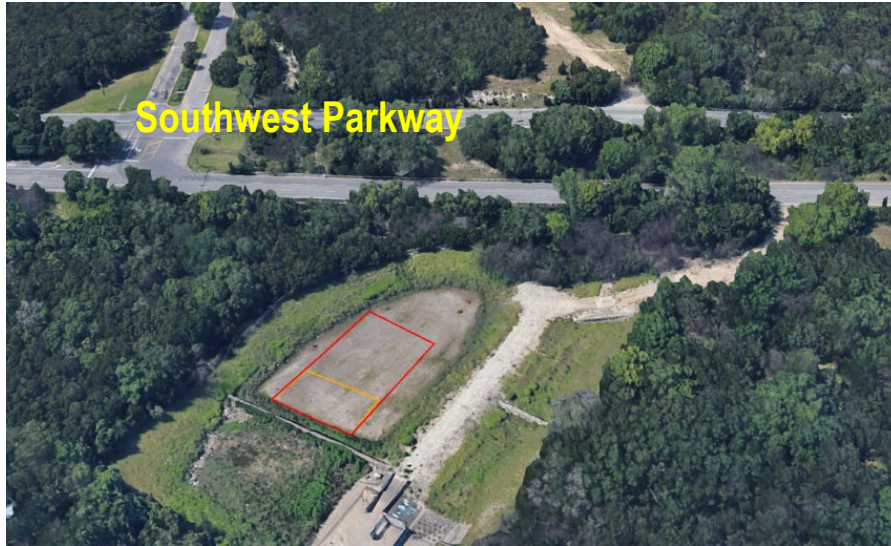
Figure 4.2: Aerial view of the Southwest Parkway (SWPW) field experiment site; the yellow rectangle is the ground surface trace of the probed volume.
