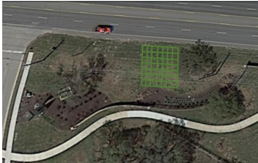
Figure 4.29: 2D FWI array at the Georgetown field experiment site; geophones are located at the grid vertices.
