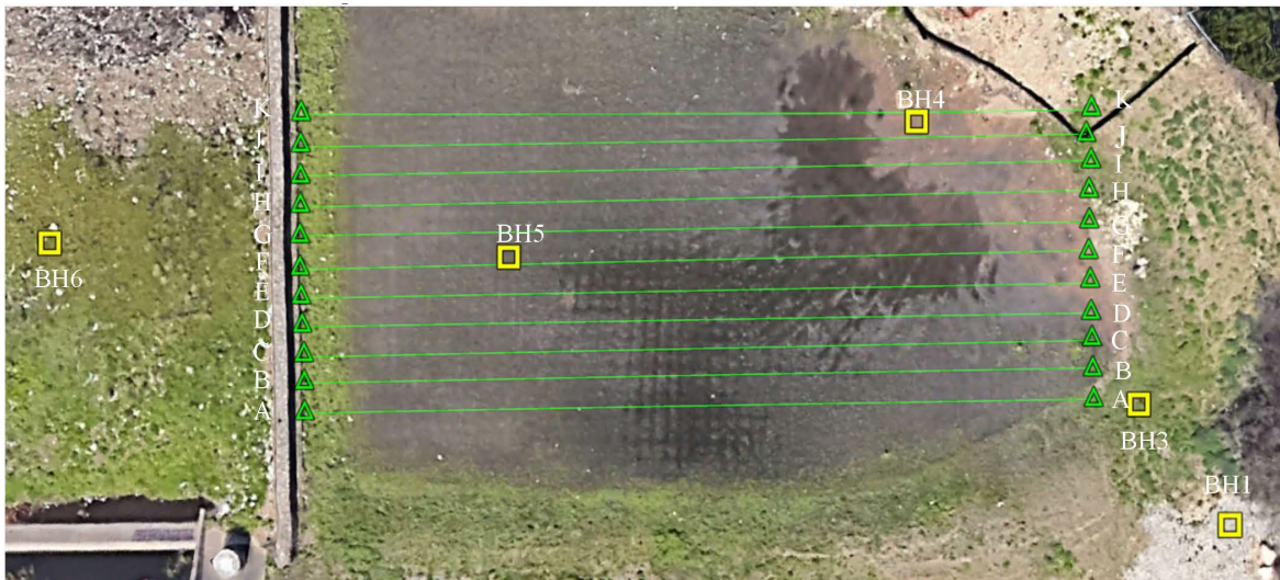
Figure 4.67: Location of boreholes relative to ERT survey lines at the Southwest Parkway site.
