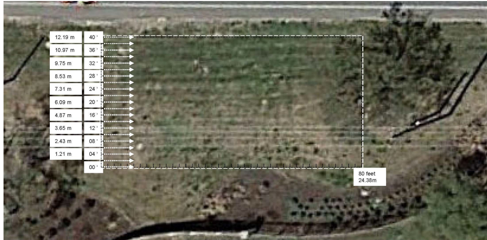
Figure 4.30: GRP scan lines at the Georgetown field experiment site.
