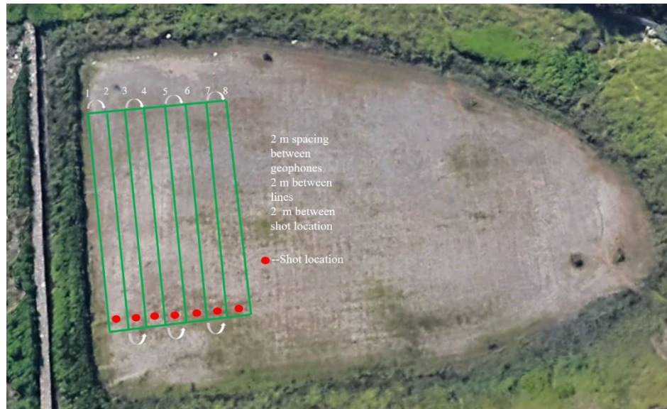
Figure 4.65: 2D FWI array at the Southwest Parkway field experiment site; geophones are located at the grid vertices.
