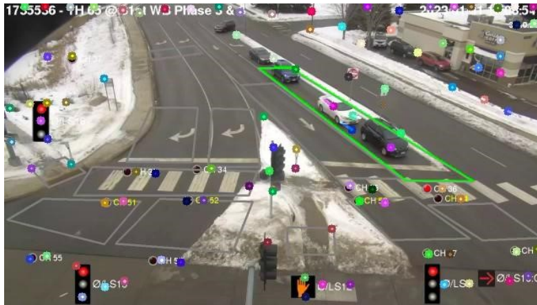
Figure 7: Results of optical flow analysis on a sequence of frames. The colored dots represent points of interest, and the colored trailing lines are the distance and direction traveled from the previous frame.
