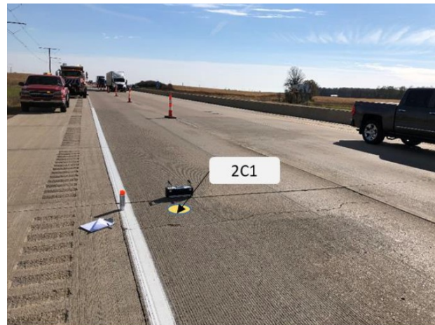
Figure 10.17 Photo and Illustration. Location of core on I-39 NB in Columbia County, Wisconsin, near a full-length transverse crack and a partial length longitudinal crack.
