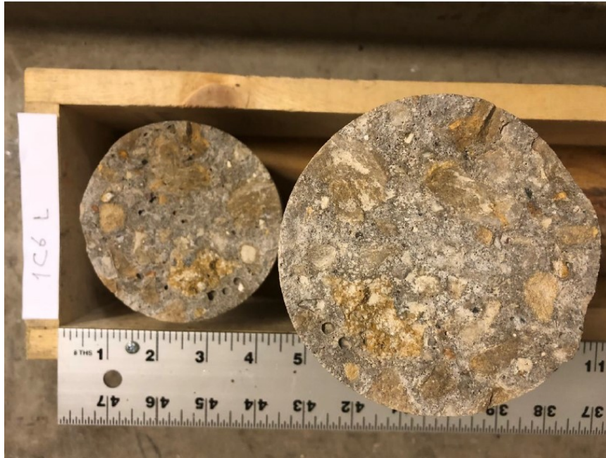
Figure 10.16 Photo. Cross section of 1C6 core from I-39 NB in Dane County, WI.
