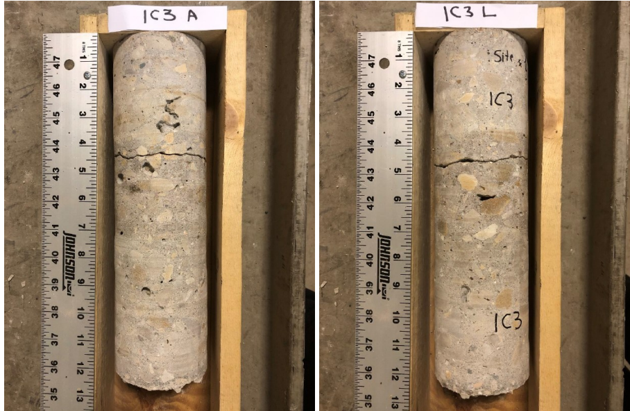
Figure 10.8 Photo. Approach side of 1C3 core (left) and leave side of 1C3 core (right) from I-39 NB in Dane County, Wisconsin.
