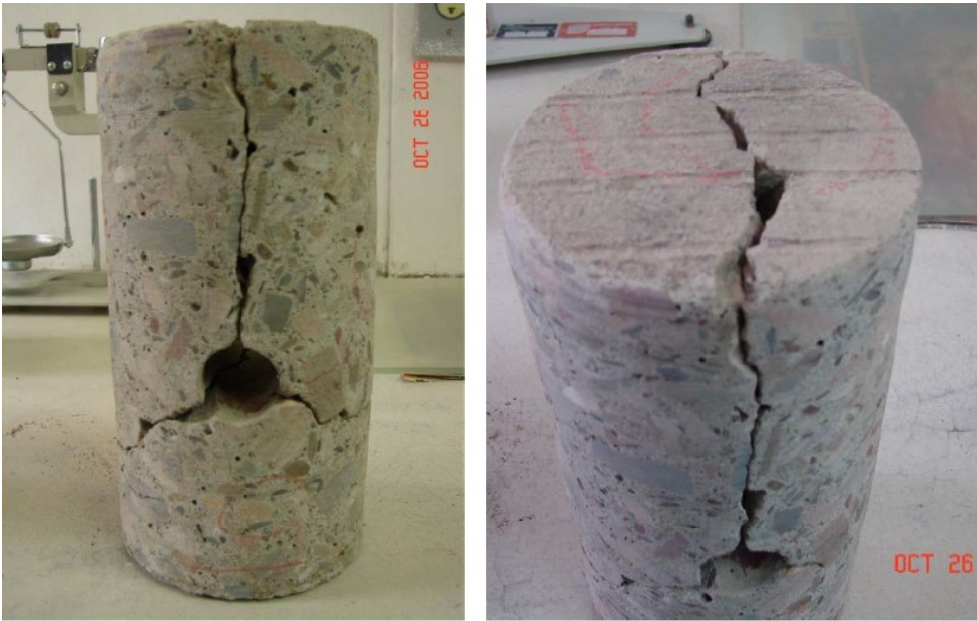
Figure 4.15 Photo. Typical cracking mode: top down.
