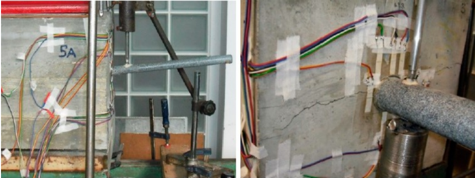
Figure 5.5 Photo. Normal stresses obtained from strain gauges; (left) beam under loading, (right) horizontal crack through the concrete beam around dowel (Zuzulova et al. 2020).
