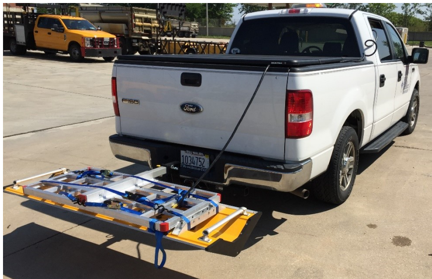
Figure 11.1 Photo. GPR system mounted to a pickup truck.
