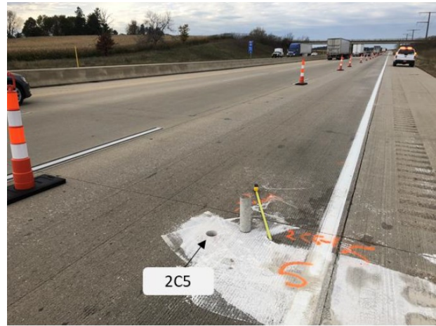
Figure 10.29 Photo and Illustration. Location of core on I-39 NB in Columbia County, Wisconsin, on a joint with no visible distresses.
