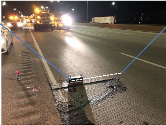
Figure 9.9 Photo and Contour Plot. 2D MIRA scan showing delamination crack initiating at dowel bar level for approach side of Joint #7 on I-94 at the Illinois Tollway.
