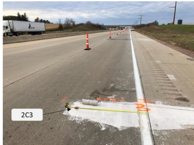
Figure 10.23 Photo and Illustration. Location of core on I-39 NB in Columbia County, Wisconsin, on concrete with no visible distresses.
