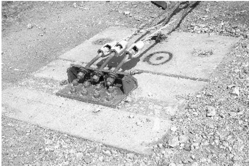
Figure 16. New York cable rail terminal after test 404211-6.
