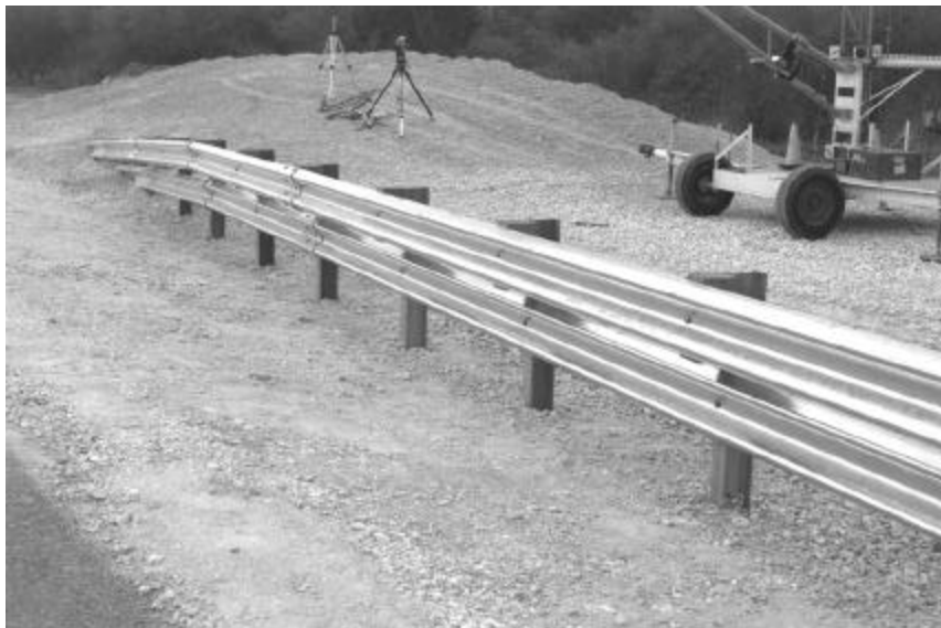
Figure 2. G4 W-beam guardrail backslope anchor terminal installation prior to test 404211-1.
