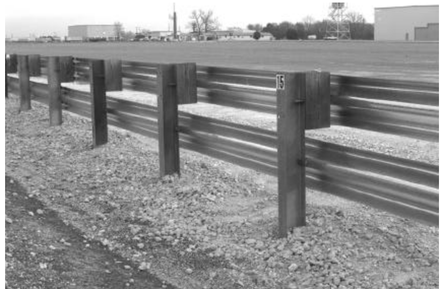
Figure 2. G4 W-beam guardrail backslope anchor terminal installation prior to test 404211-1.
