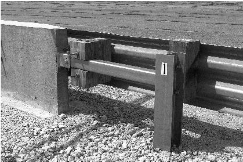
Figure 43. Nebraska thrie beam transition prior to test 404211-7.
