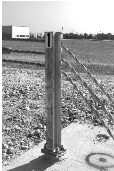
Figure 14. New York cable rail terminal installation prior to test 404211-6.
