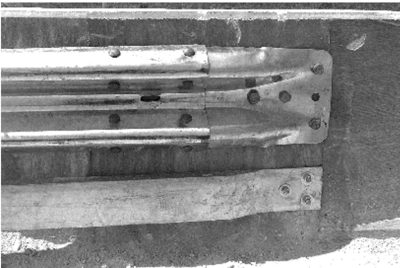
Figure 31. Vertical flared back transition prior to test 404211-4.
