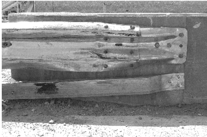
Figure 33. Installation after test 404211-4.
