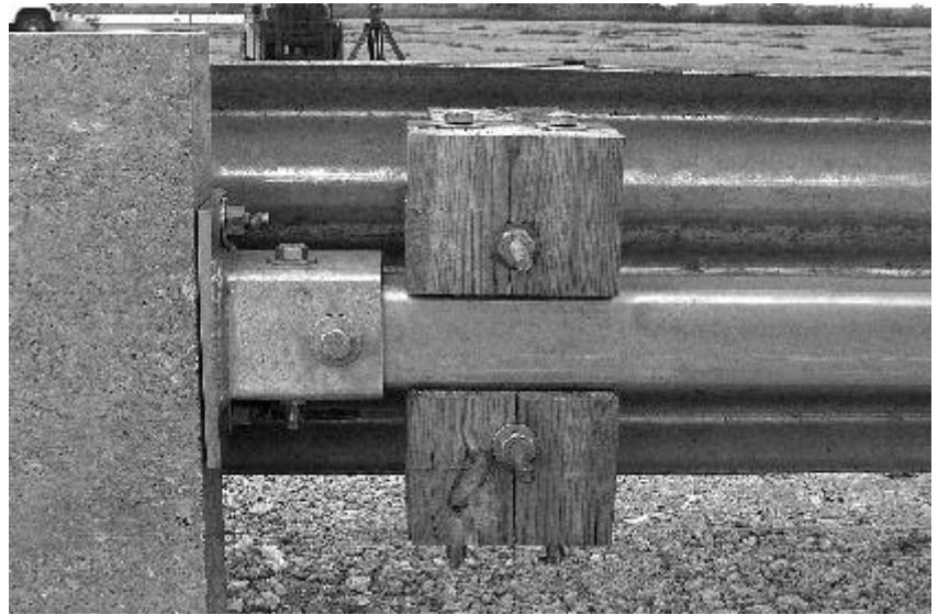
Figure 43. Nebraska thrie beam transition prior to test 404211-7.
