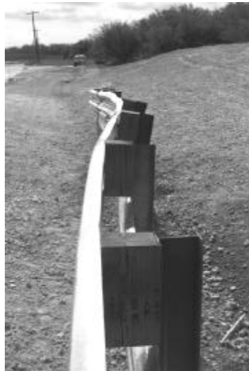
Figure 4. G4 W-beam guardrail buried-in-backslope terminal after test 404211-1.
