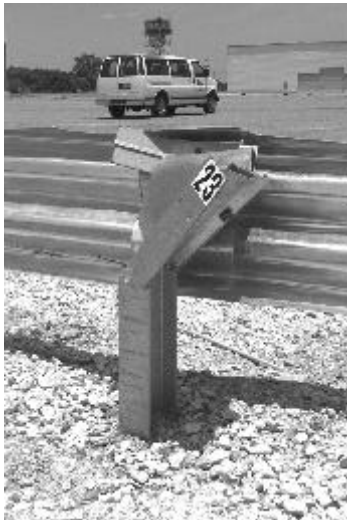
Figure 76. Installation after test 404211-5.
