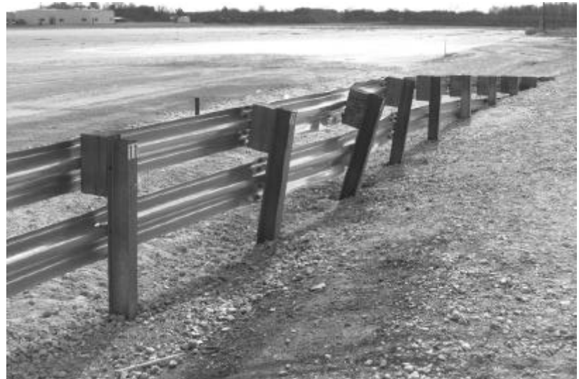
Figure 4. G4 W-beam guardrail buried-in-backslope terminal after test 404211-1.
